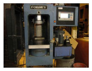
Figure V.10. EAC-3 cylinders were broken every hour from 5 to 10 hours, at 24 hours, and at 72 hours.
