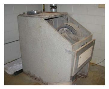
Figure T.5. Jaw crusher used to produce I-94 laboratory-crushed RCA.
