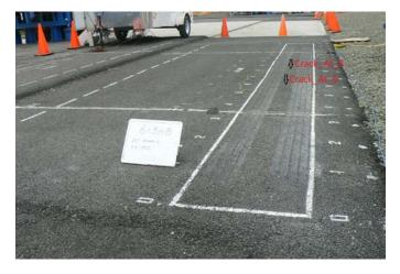
Figure K.12. Section photograph at test completion for Section 613HB, along with labels for cracks.
