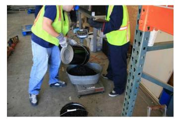
Figure G.49. Weighing of hot HMA for placement into ingot molds.
