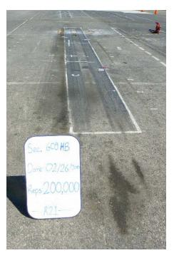
Figure L.20. Photograph at test completion of Section 609HB, PG 64-28 PM, 114 mm.
