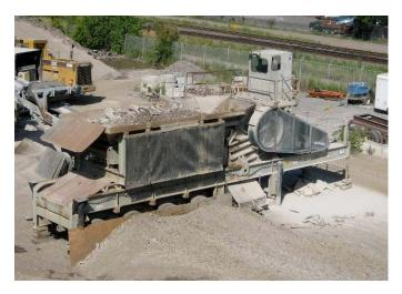
Figure F.9. The primary crusher was the jaw crusher operating at less than full capacity.
