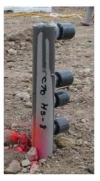
Figure H.8. Concrete relative humidity sensors installed in Cell 70.
