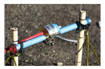
Figure G.19. Static strain gauge affixed to aggregate base with wire fixtures.
