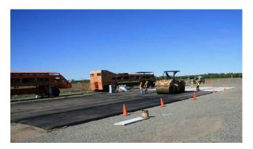
Figure G.47. Completed test track showing two HMA lift thicknesses and PCC sections.
