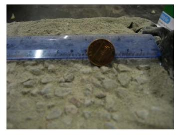
*Figure V.4. Shows approximate depth of etch between 3 and 5 mm.*
