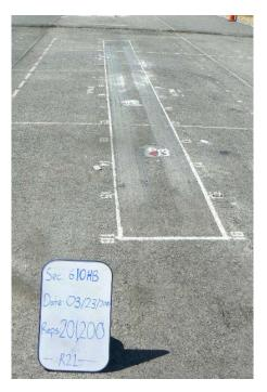
Figure L.31. Photograph at test completion of Section 610HB, PG 64-28 PM, 64 mm.
