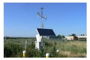
Figure M.2. Photograph of the automatic datalogging weather station at the project site.
