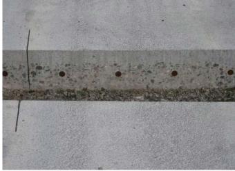
Figure F.28. Cross section of the PCC/PCC demonstration slab constructed at MnROAD showing very good integrity and bond between the two PCC layers.
