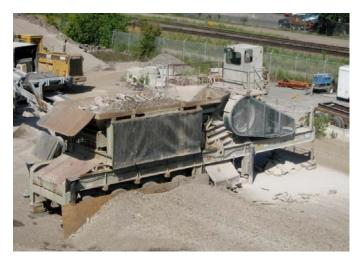
Figure T.3. Jaw crusher used in the production of limestone industrial and I-94 industrial RCA.
