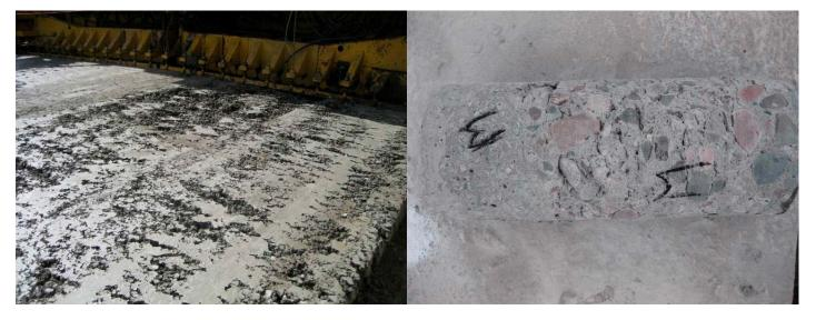
Figure F.26. At left, "torn" edges and surface caused by concrete setting on various parts of the paver; at right, coring showed poor mix consolidation in the lower PCC at select locations.
