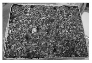
Figure U.3. Scaled test surfaces of an EAC concrete sample after 56 freeze-thaw cycles.
