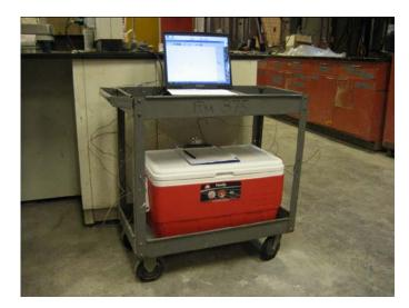
Figure V.9. Concrete temperature data acquisition system.
