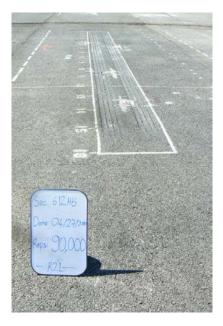
Figure L.52. Photograph at test completion of Section 612HB, RHMA-G, 64 mm.
