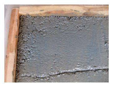
Figure V.13. There is not enough paste available to close the surface of the EAC field sample.
