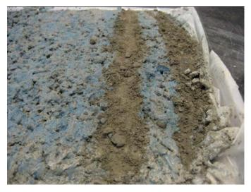
Figure V.6. EAC-2 concrete specimen with curing/ retarder BASF MBT Reveal. Scratches at 2 and 3 hours show that aggregate is easily removed from paste.
