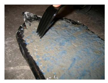
Figure V.3. Brushing readiness test at 5 hours.
