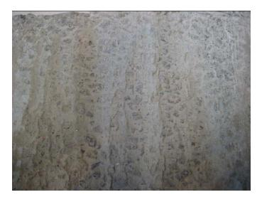
Figure V.8. Surface of revised EAC concrete specimen at 7 hours.
