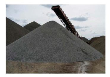
Figure F.31. RCA stockpile being processed and saturated at a concrete recycling facility.
