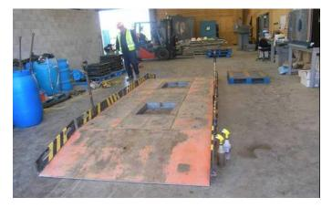
Figure G.48. Assembled compaction frame and ingot molds for field mix-lab compact HMA specimens.
