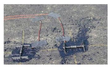
Figure G.44. Sensors placed on bottom lift of PG 64-28PM, glued with mastic of sand and emulsion.
