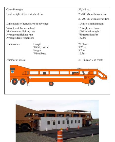
Figure L.5. Specifications and photograph of HVS on SHRP 2 R21 test section at UCPRC.
