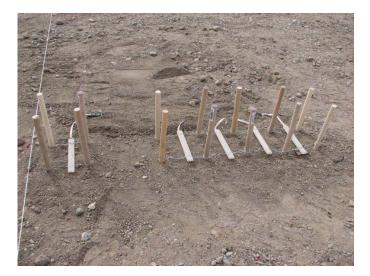
Figure H.15. Dynamic strain gauge installation for Cells 71 and 72.
