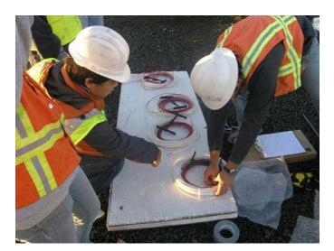
Figure G.42. CTL strain gauges, with 30 feet of coated cabling for thermal protection.
