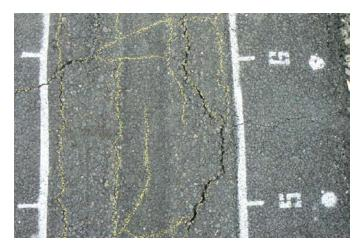
Figure K.92. Section 614HB: Top view of the section between Stations 5 and 6 after completion of HVS testing. Transverse cracks (i.e., running left to right) can be seen. Chalk lines indicate hairline cracks visible at the pavement surface.
