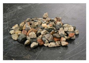
Figure T.8. I-94 industrial crushed RCA wetted to distinguish natural aggregate from residual mortar.
