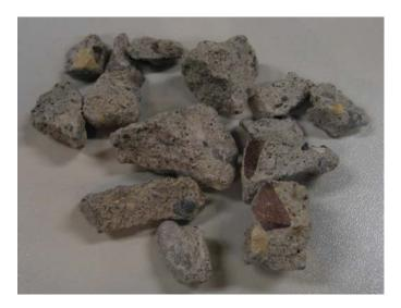
Figure Q.3. Laboratory-crushed RCA.
