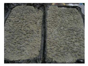
Figure V.5. Specimens with Sika Rugasol-S (at left) and BASF MBT Reveal (at right) after brushing.
