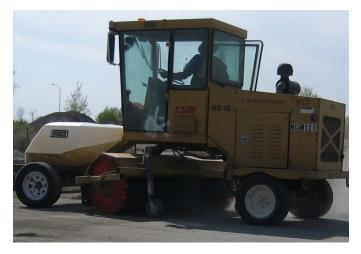
Figure V.17. Rotating sweeper brush with mechanical arm extended to relieve pressure on the brush.
