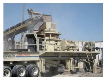
Figure F.10. Cone crusher was used as secondary crusher to further remove the mortar from the natural aggregates.
