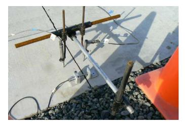
Figure M.3. Photograph showing the JDMD configuration for monitoring both horizontal and vertical movements at a joint. The horizontal JDMD shown is model DSD800SE5 made by Daytronic, and the vertical JDMDs are model GHSD/GHSDR 750 made by Macro Sensors.
