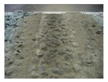
Figure V.7. At 6 hours, the mix could be brushed and aggregates exposed without dislodging from the paste.
