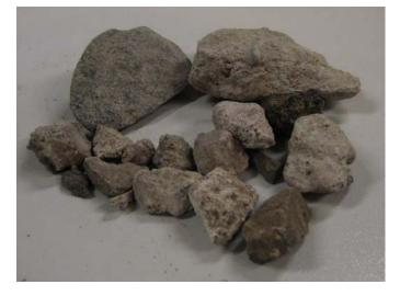
Figure Q.2. Minneapolis RCA that originated from multiple sources.
