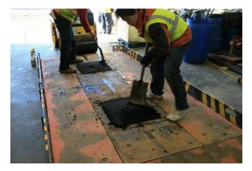
Figure G.50. HMA mix being spread out in the mold.
