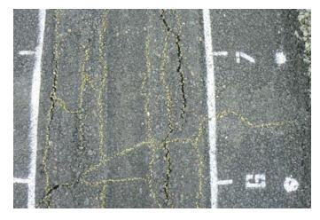
Figure K.93. Section 614HB: Top view of the section between Stations 6 and 7 after completion of HVS testing. Transverse cracks (i.e., running left to right) can be seen. Chalk lines indicate hairline cracks visible at the pavement surface.
