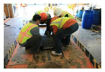
Figure G.52. Removal of compacted HMA ingot, with a weight of approximately 150 lb.
