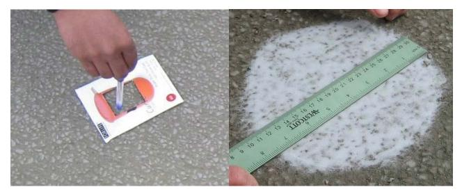
Figure F.36. Quality control tests for brushing: (left) 25 cm<sup>2</sup> test to count aggregate peaks, and (right) sand patch test to determine texture depth.
