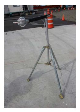
Figure M.4. Photograph of NovaLynx 240-8104 Albedometer (Dual Pyranometer) used for albedo measurement.
