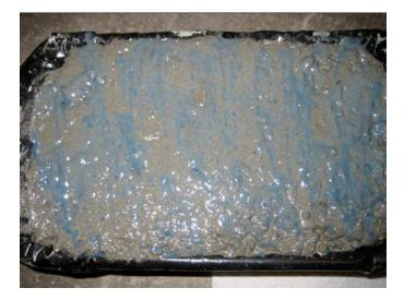
*Figure V.1. Specimen with BASF MBT Reveal surface treatment.*
