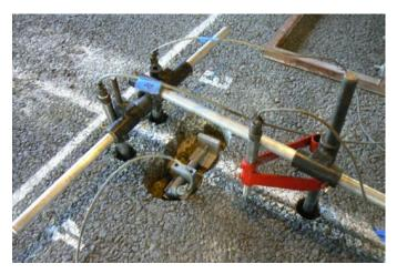
Figure K.6. Photograph shows JDMDs installed at traffic side (inner slab) near Joint J4. There are two vertical JDMDs on PCC, one horizontal JDMD on PCC, and one vertical JDMD on HMA.
