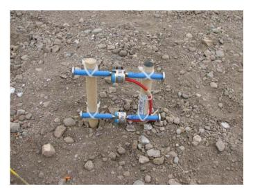
Figure H.10. Static strain gauge installation for Cell 70.
