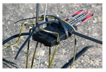
Figure G.20. Moisture sensor in place before PCC placement.
