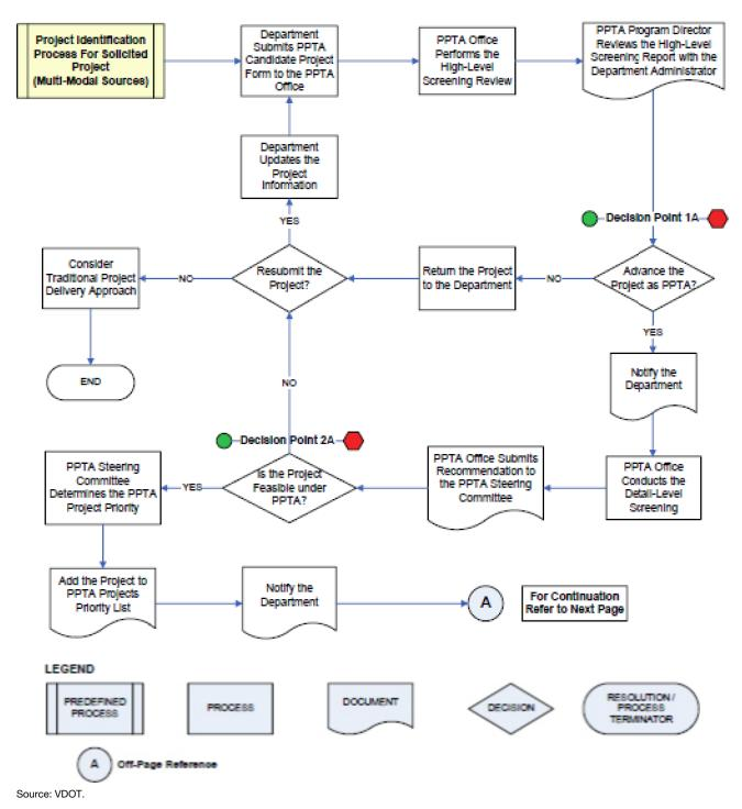
Figure B.1a. Virginia PPTA Implementation Manual and Guidelines: Project Delivery Framework Flowchart (Solicited Projects).
