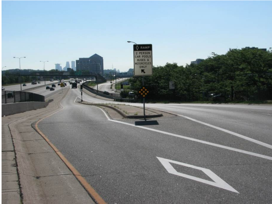
Figure 72. Queue Jump Lane on Metered Ramp in Minnesota (4)
