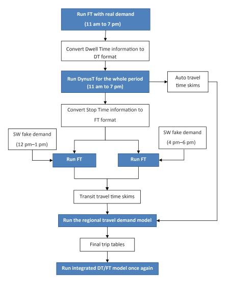
Figure 5.8. The DynusT–FAST-TrIPs integration framework.
