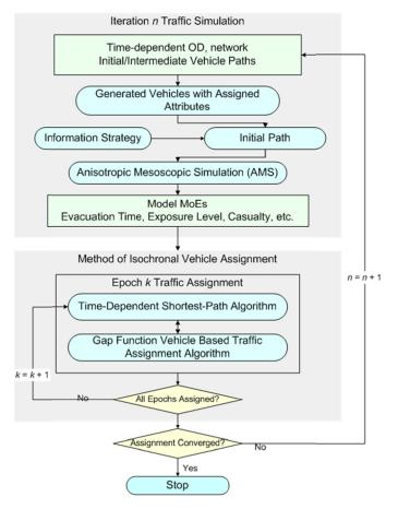
Figure 2.1. DynusT model algorithmic structure.
