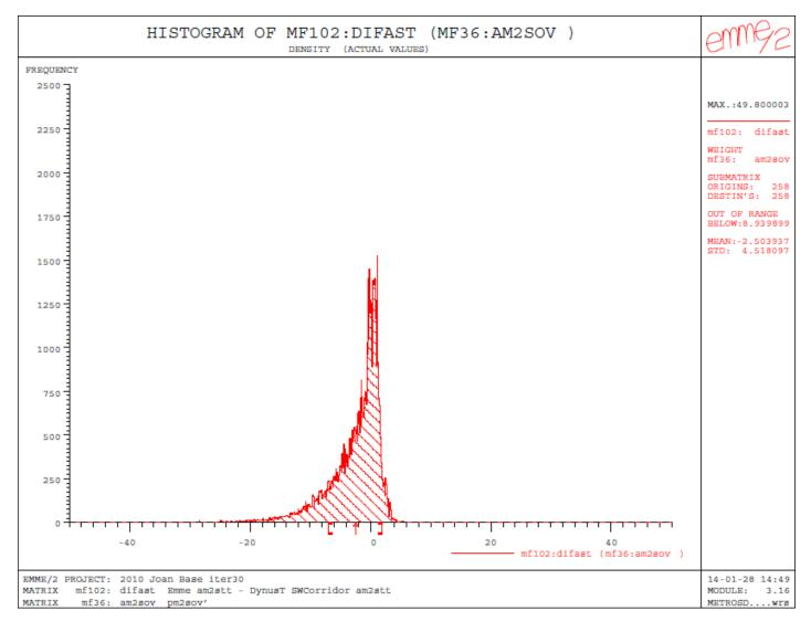
Figure 5.9. Difference in AM peak-period SOV automobile travel times for Southwest Corridor zone pairs (weighted by trips): mean = -2.5 min, standard deviation = 4.5 min.
