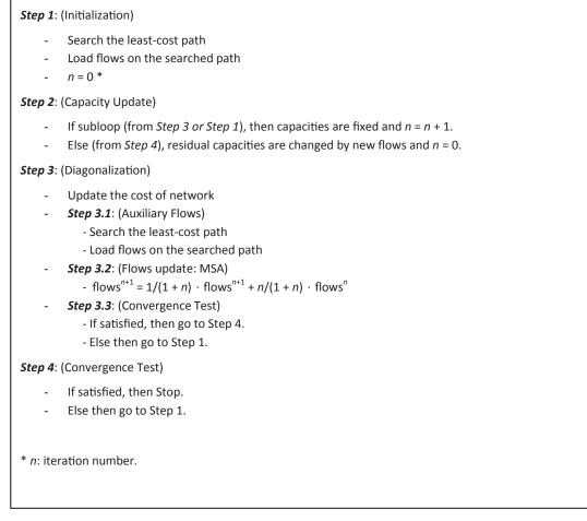
Figure 2.5. Transit assignment algorithm, using diagonalized method of successive averages (MSA) with hyperpath.
