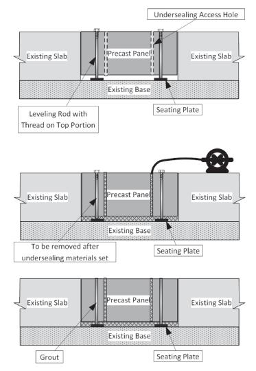
Figure 10.5. Panel placement using threaded setting bolts.
