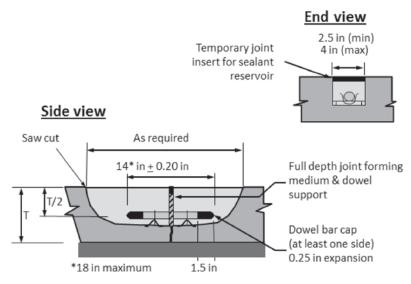
Figure 5.5. Dowel bar retrofit features.
