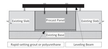
Figure 10.4. Panel placement using strongback beams.
