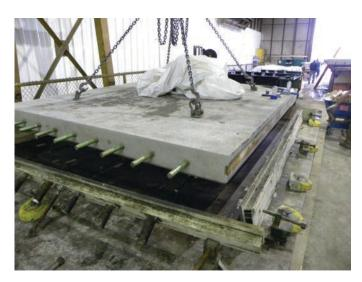
Figure 9.9. Stripped panel being moved to another location and panel with project-specific markings.
