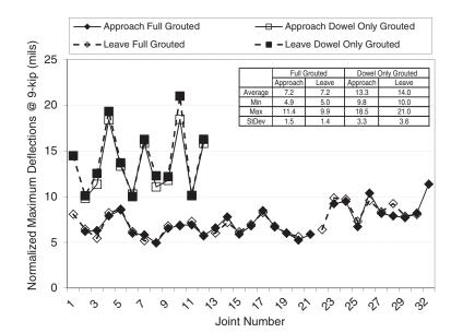
Figure 3.14. Normalized maximum deflections for joint testing of I-15 JPrCP project in California.
