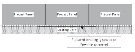
Figure 11.3. Panel placed directly on prepared bedding over existing base.
