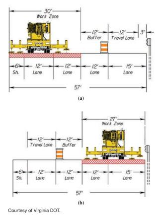
Figure 15.7. Crane footprints for I-66 PPCP project for panel placement in (a) inside two lanes and (b) outside two lanes.
