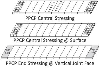
Figure 2.8. Schematic of three PPCP systems.
