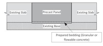
Figure 10.3. Panel placed directly on prepared bedding over existing base.
