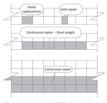
Figure 2.1. Applications of PCP for (top) localized, (center) short-length, and (bottom) continuous repair.
