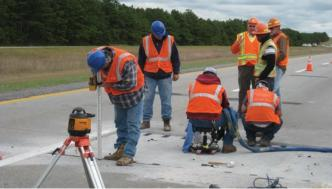
the performance of the two test sections as they are subjected to aircraft loadings.
