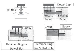
Figure 14.7. Steps for installing dowel bars in narrow-mouth dowel slots.
