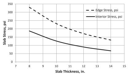
Figure 8.4. Stresses as a function of panel thickness.
