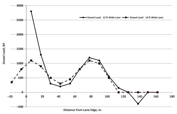
Figure 5.1. Load transfer along a joint.
