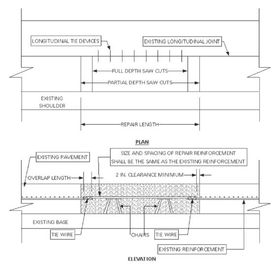
Figure 14.2. Continuity of longitudinal steel within the FDR area.
