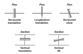
Figure 5.3. Types of dowel bar misalignment.
