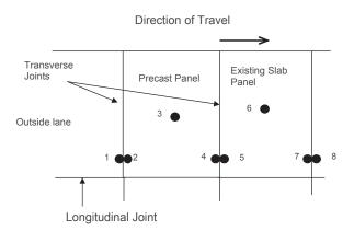
Figure C.1. FWD test locations for jointed systems.
