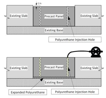
Figure 10.6. Panel placement using polyurethane foam.
