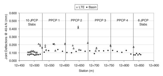
*Figure 3.20. Average deflections at transverse joints with a 9,000-lb (40.0-kN) load level.*
