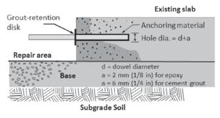
Figure 5.4. Epoxy-grouted dowel bar anchoring in a drilled hole.
