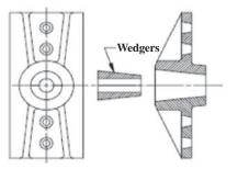
Figure 7.1. Monostrand anchorage system.
