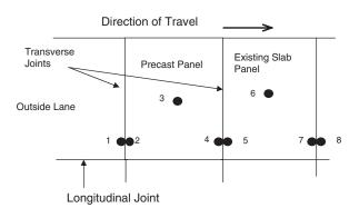
Figure 3.1. FWD test locations for jointed systems.
