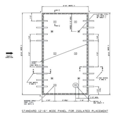
Figure 2.13. Illinois Tollway intermittent repair system.
