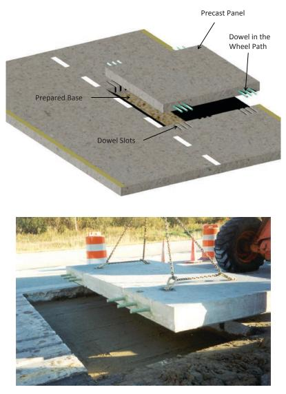
Figure 2.3. Variation of intermittent repair technique with slots for dowel bars cut in existing concrete pavement.
