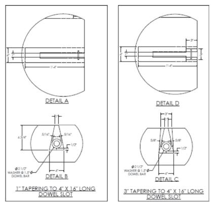
Figure 14.9. Details of the standard slot and of the standard slot with wider opening at the joint face.
