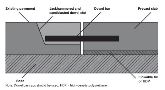
Figure 2.2. Schematic of intermittent repair application.
