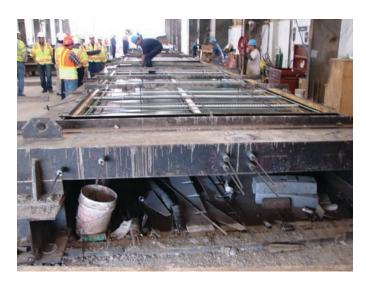
Figure 9.8. Pretensioning process.
