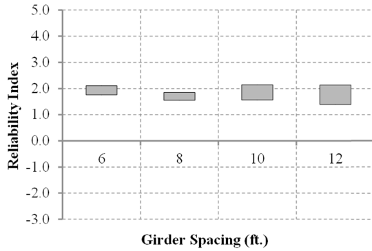
Figure 6.26. Reliability indices of various bridge decks designed using a 1.0 live load factor over a 1-year return period (ADTT = 5,000) for positive moment region, Class 1 exposure.
