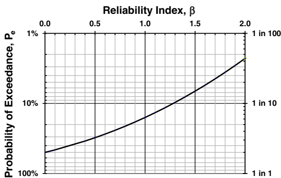
Figure 6.20. Relationship between \beta and P_e for the case of a single load and single resistance.
