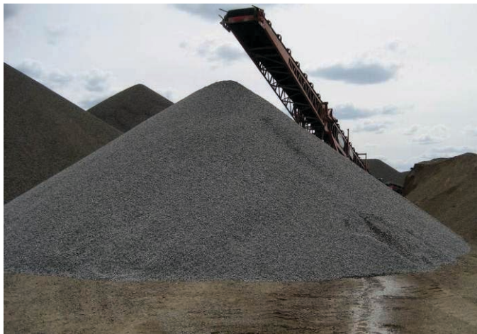
Figure 2.20. RCA stockpile being processed and saturated at a concrete recycling facility.
