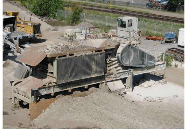
Figure 2.7. The primary crusher was the jaw crusher operating at less than full capacity.
