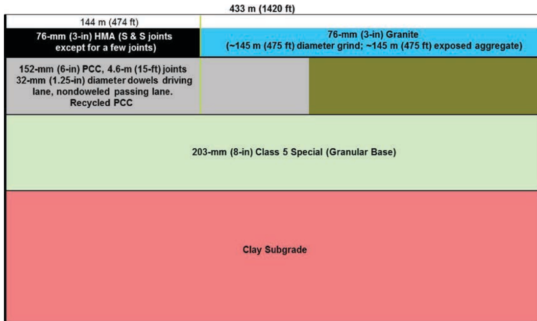
Figure 2.4. Layout of test sections at MnROAD (Cell 70, HMA/PCC; Cell 71, PCC/RCA PCC; Cell 72, PCC/low-cost PCC).
