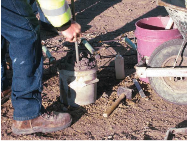
Figure 5.3. QA testing of the PCC layer for entrained air and slump.
