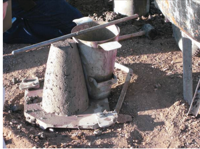
Figure 5.3. QA testing of the PCC layer for entrained air and slump.
