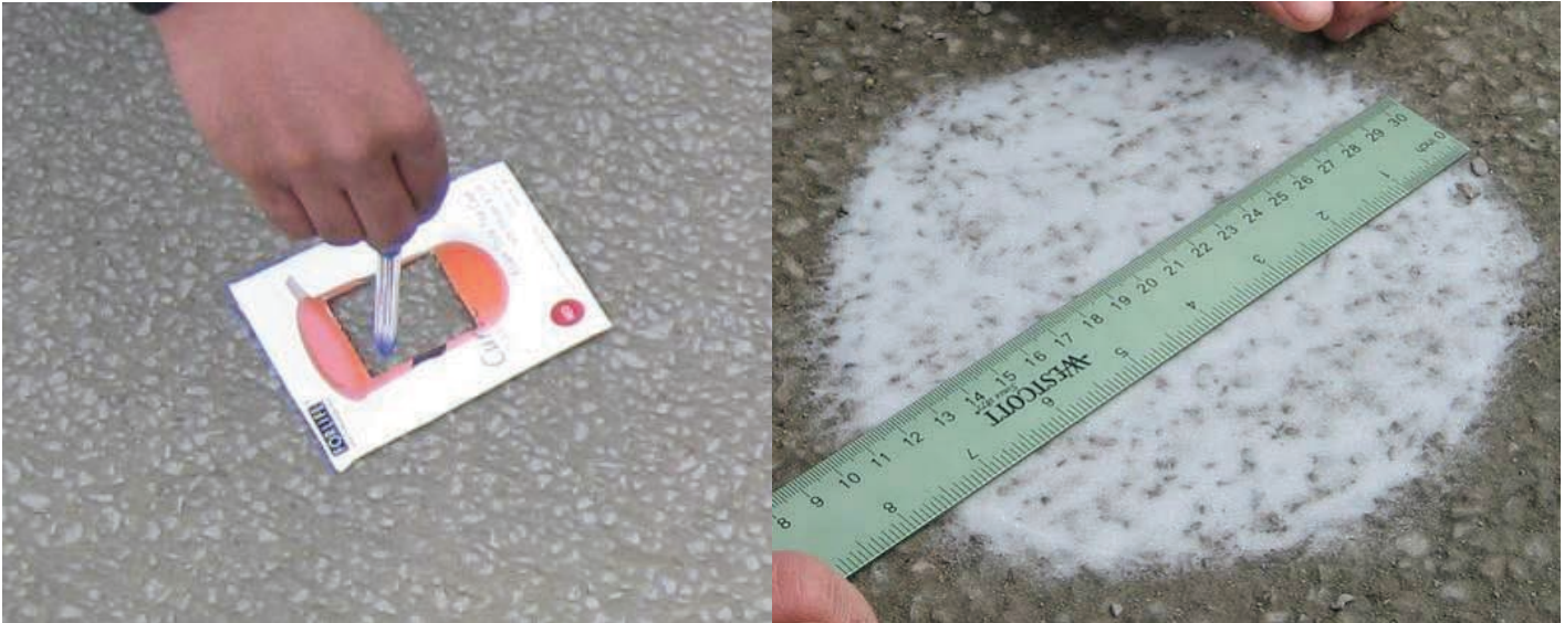
Figure 2.25. Quality control tests for brushing: (left) 25 cm 2 test to count aggregate peaks and (right) sand patch test to determine texture depth.
