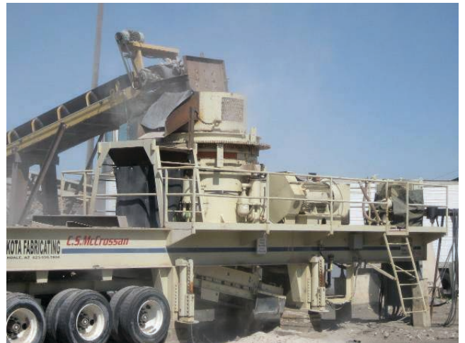
Figure 2.8. A cone crusher was used as a secondary crusher to further remove the mortar from the natural aggregates.
