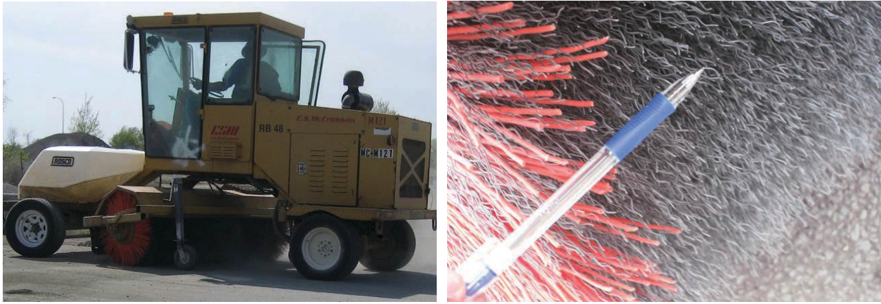
Figure 5.9. Rotating sweeper brush with mechanical arm extended to relieve pressure on the brush (left) and close-up of the brush bristles (right).
