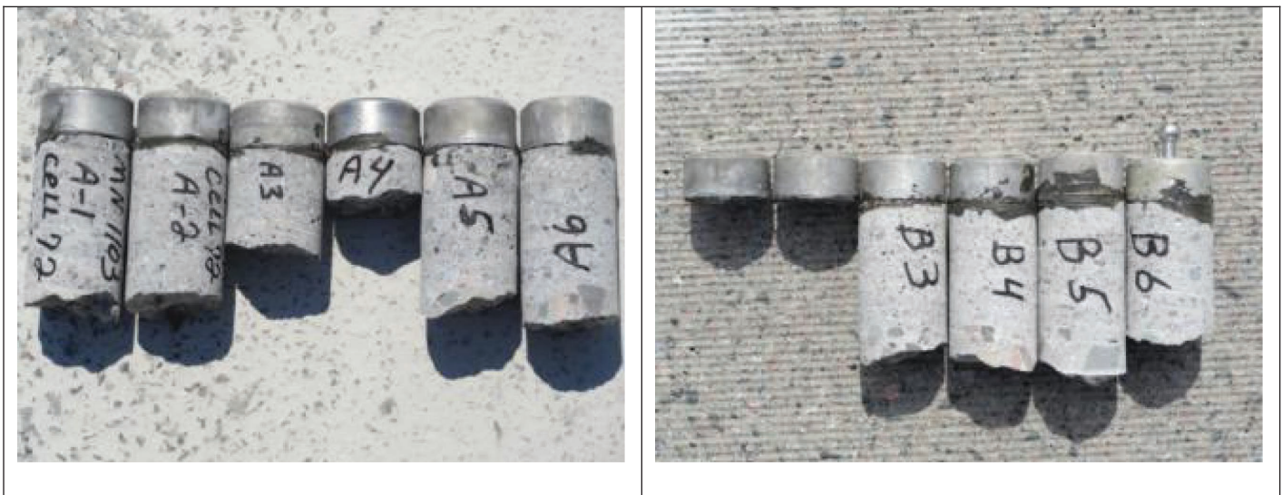
Figure 3.33. Fractured cores: Cell 72 (left) and Cell 71 (right).
