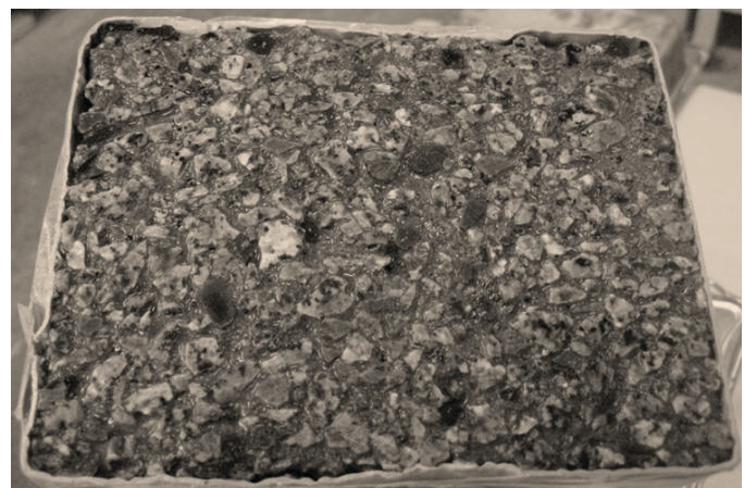
Figure 3.12. Scaled test surfaces of an EAC sample after 56 freeze–thaw cycles.
