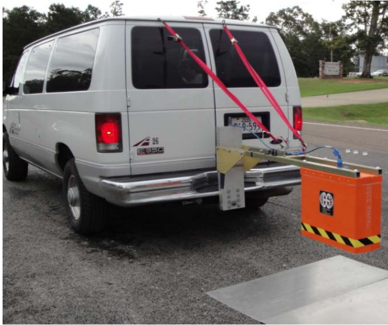
Figure 5.1 Air Coupled GPR systems for highways. (Photo: Tom Scullion)
