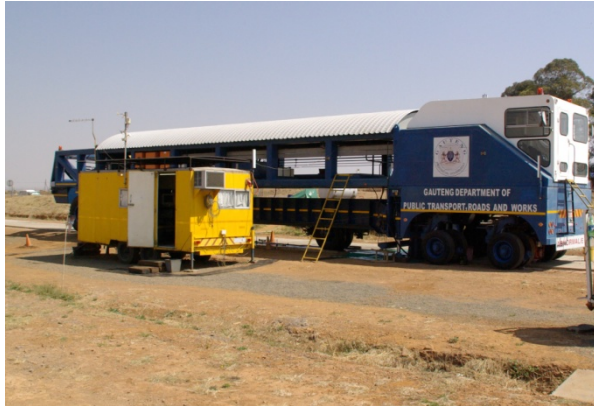
Testing of thin CRCP near Heidelberg, South Africa.
