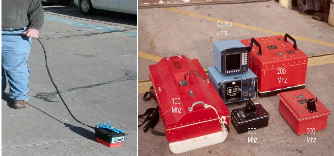
Figure 5.2 Ground coupled systems, 1.5 GHz on left, lower frequency antennas with control unit on right. (Photos: Tom Scullion)
