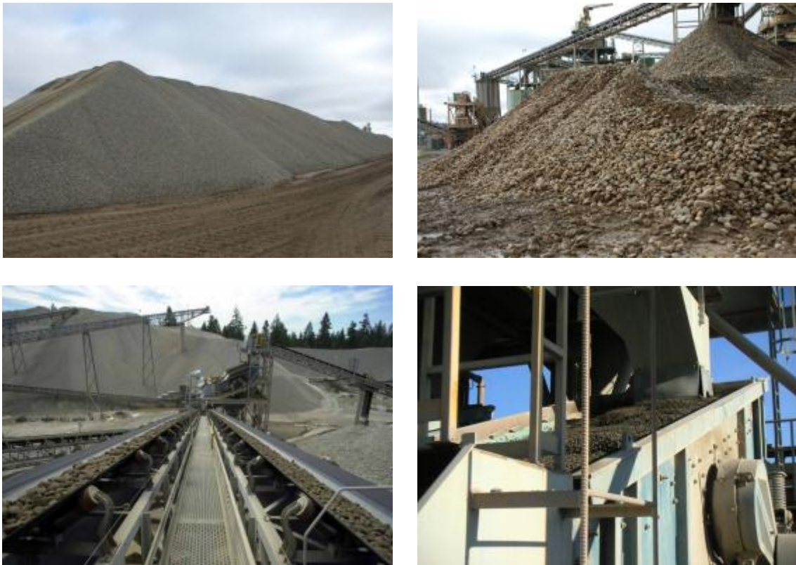
Figure 14. Aggregate processing, which includes stockpiles, conveyors, and screening. (Photos: Joe Mahoney)
