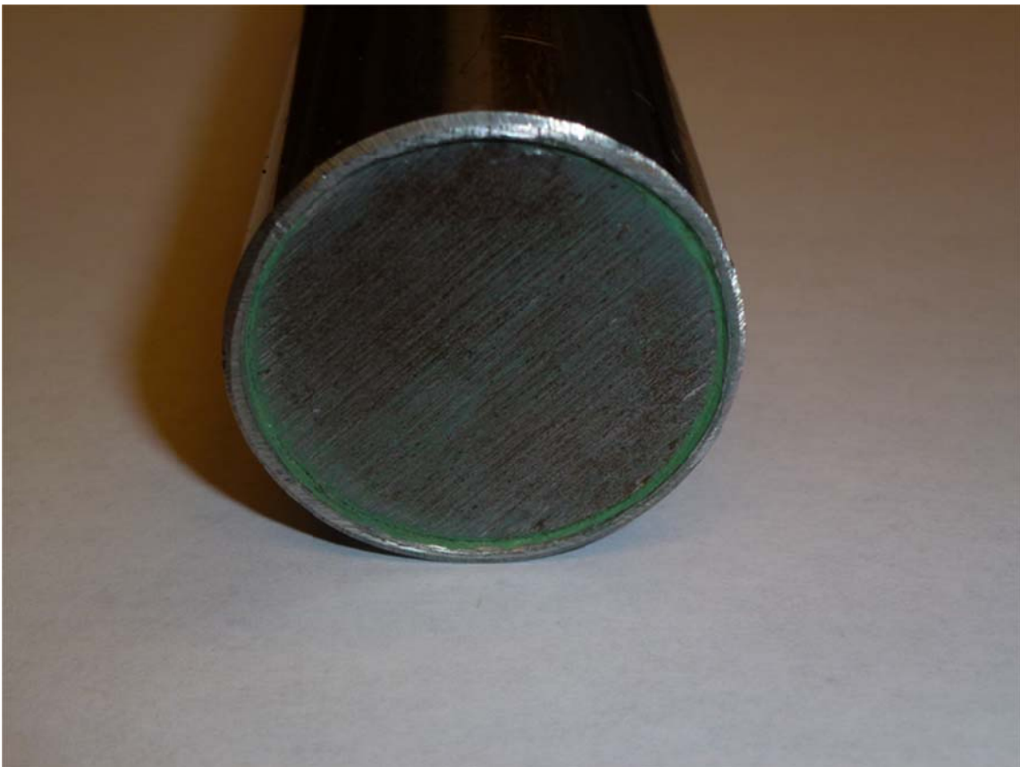
Figure 20. Stainless dowel bar. (Photo: Joe Mahoney)
