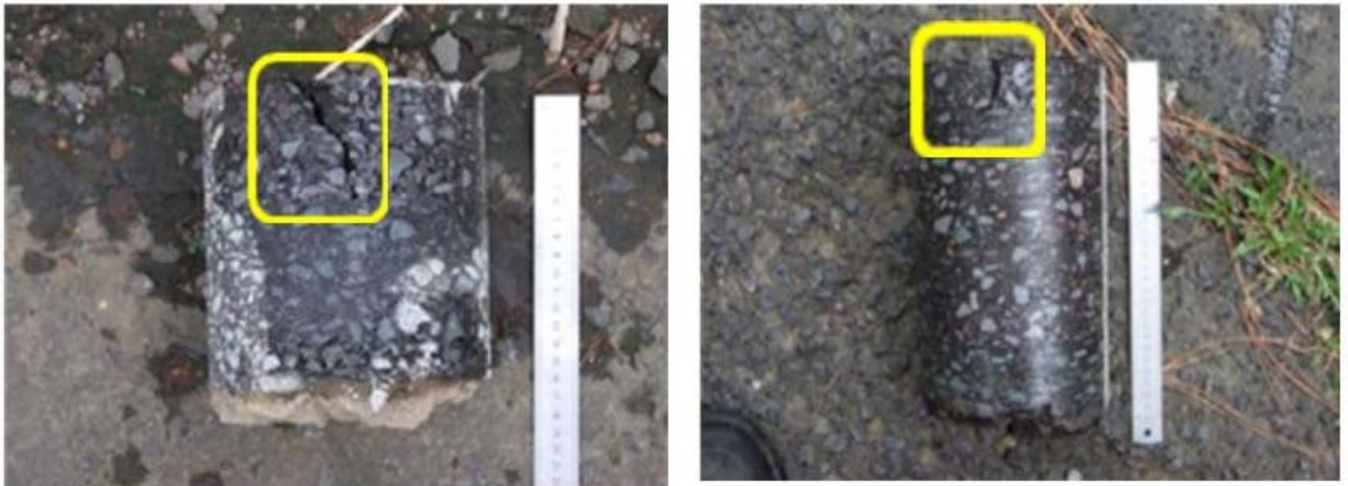
Figure 27. Top down cracking in cores from Panama. (core thicknesses ranged from 6 to 12 in. thick)
