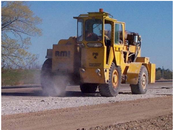
(a) Resonant breaker machine (Photo: Karim Chatti)
