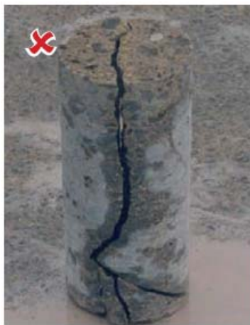
(c) Non-compliant core: Over-cracked
