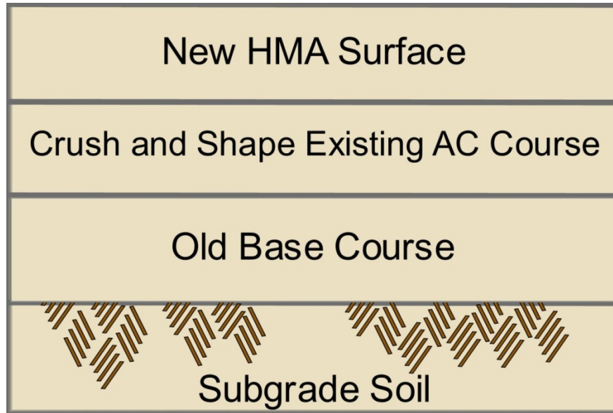
Figure A.2. Schematic of a HMA over a crushed and shaped HMA pavement.
