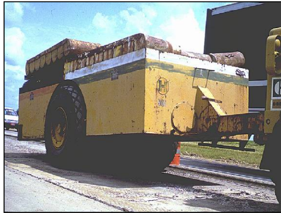
Figure A.6. Heavy roller used to seat the cracked pavement. (NHI, 2003)
