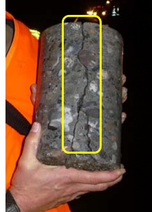
(f) Compliant crack illustrated by reassembled core
