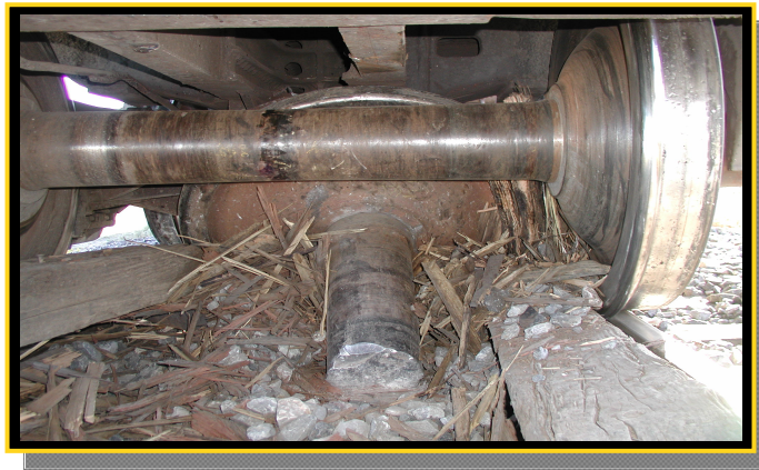
Figure 1: Broken railroad axle
