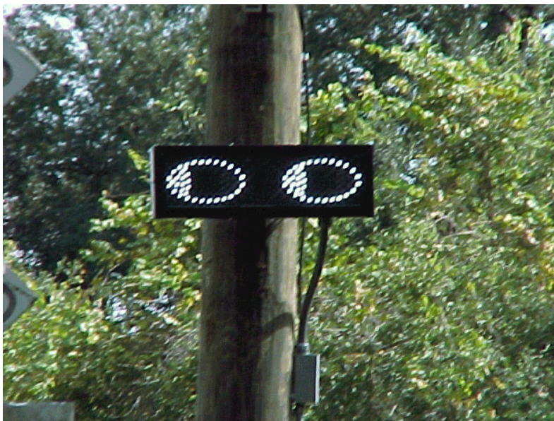
Figure 7, Animated 'eyes' signal used in this rail crossing experiments.
