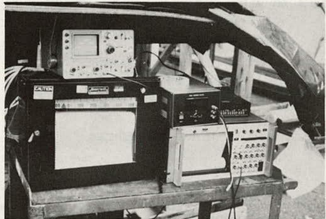
Figure 7. Setup for determining radiometer performance during outdoor engineering development tests. Shown are thermocouple recorder, radiometer internal calibration waveform, and radiometer temperature indicator and recorder.
