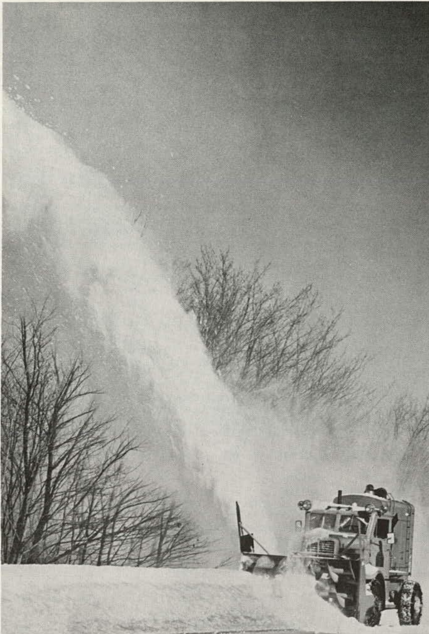
Figure 4. Rotary Plow Dispersing Windrow Formed by V-Plow.
