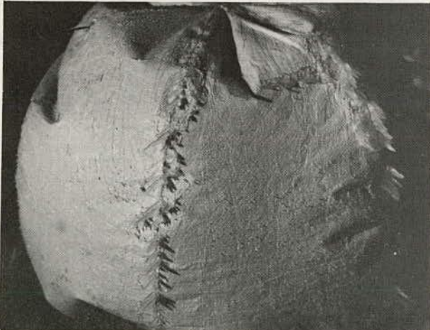
Figure 11 De-icing by inflation of a soft plastic sheet covering a spherical radome
