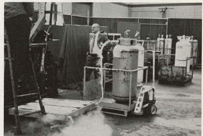
Figure 10. Preliminary engineering test of radiometric measurement of the temperature of frost and ice on an artificially cooled asphalt test slab.
