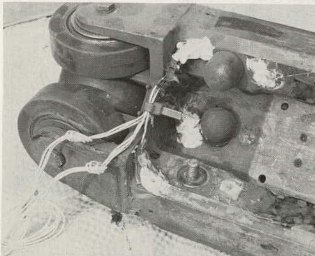
FIGURE 9: PRESENT POWER COLLECTOR/HEATING WIRES
