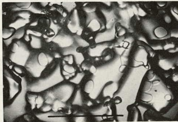
Figure 10. Dry snow grains in contact with a glass plate. Mirror-like contact plane surfaces are seen. Scale: 1mm.
