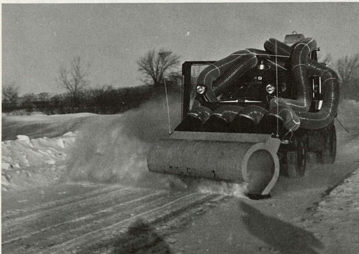
Figure 6. MK 2 air lubricated snow plow in road service.
