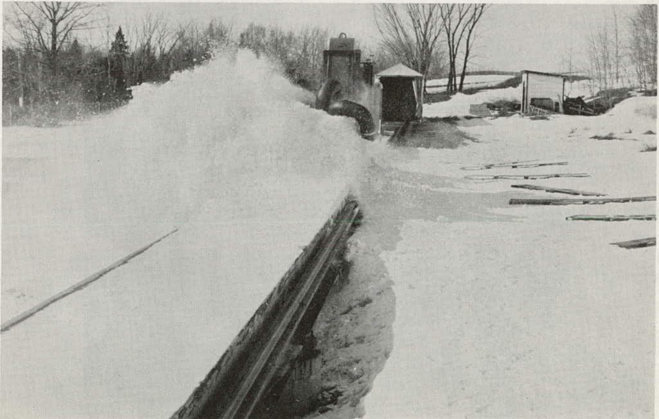
Figure 4. MK 1 air lubricated snow plow at approximately 15 km/h.
