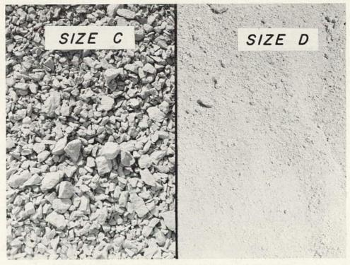
Figure 72. Aggregates for crushed stone base course, special.
