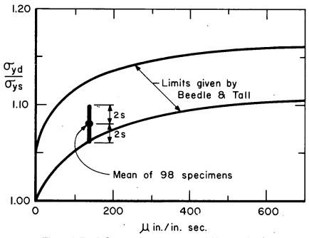
Figure 2-E. Influence of strain rate on yield stress level.
