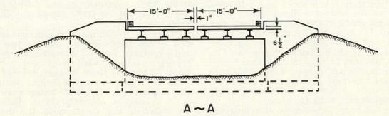
Figure 26. Typical bridge sections.
