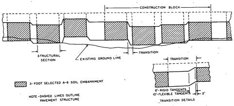
Figure 9. Typical longitudinal section of embankment of test tangents.
