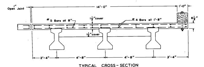
Figure 126. Prestressed concrete beam bridges.
