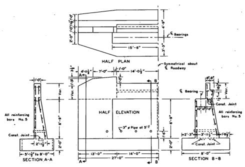
Figure 118. Typical abutment.
