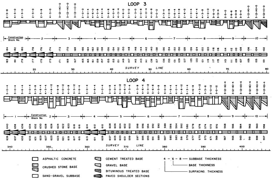
Figure 13. Layout of flexible tangent, Loops 3 and 4.
