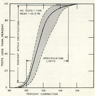
Figure 79. Crushed stone base compaction.
