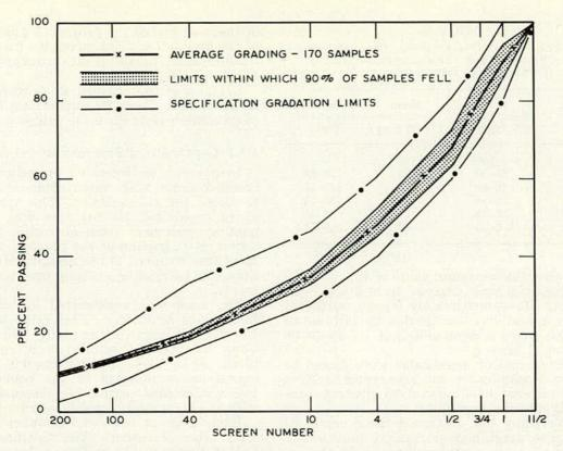
Figure 73. Gradation of crushed stone base, special-plant samples.
