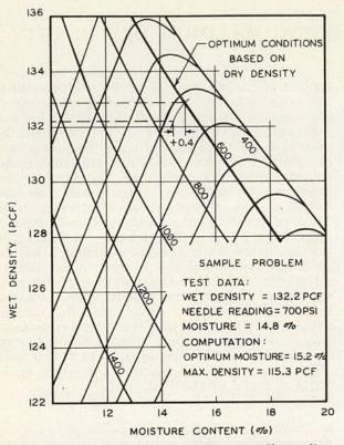
Figure 2-B. Moisture-density-Proctor needle reading curves.
