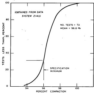
Figure 90. Bituminous-treated base course compaction.
