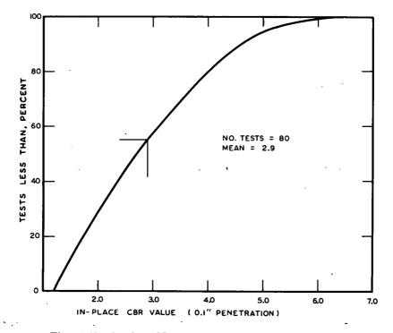
Figure 49. In-place CBR determination of embankment on flexible tangents at time of paving.
