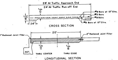
Figure 122. Bridge approach slabs.
