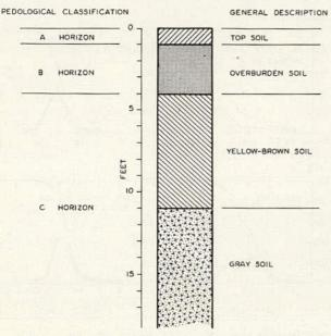
Figure 28. Typical boring log from borrow pit.
