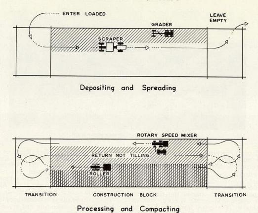
Figure 38. Equipment operation on embankment.
