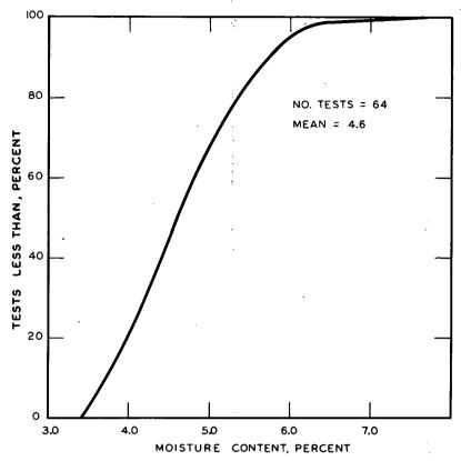
Figure 70. Subbase moisture content on flexible tangents after paving.
