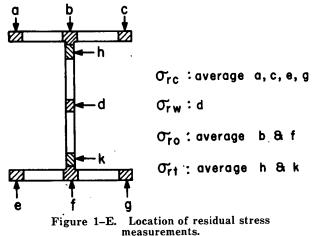
was cut out, and again after the section was cut into strips. The 2-ft beams were sectioned into ½- by 11-in. strips after the initial readings were taken; a second set of readings was taken on the strips.
