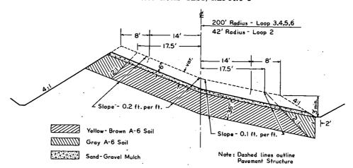
Figure 10. Typical cross-section of embankment on turnarounds with sand-gravel mulch cover.
