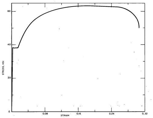
Figure 142. Typical stress-strain curve for structural steel.
