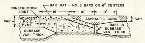
Figure 24. Details of transitions between rigid and flexible pavements.
