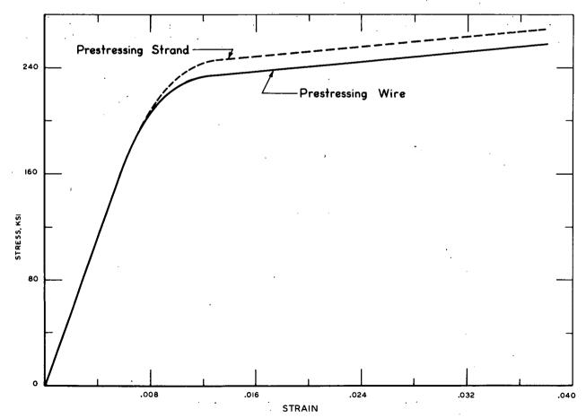
Figure 143. Typical stress-strain curve for prestressing steel.
