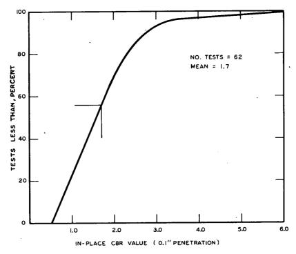
Figure 50. In-place CBR determination of embankment on rigid tangents at time of paving.
