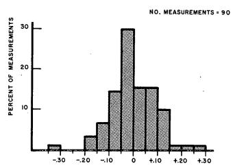
VARIANCE FROM MEAN MEASURED DIMENSIONS, INCHES Figure 149. Measurements of slab thickness, all bridges.
