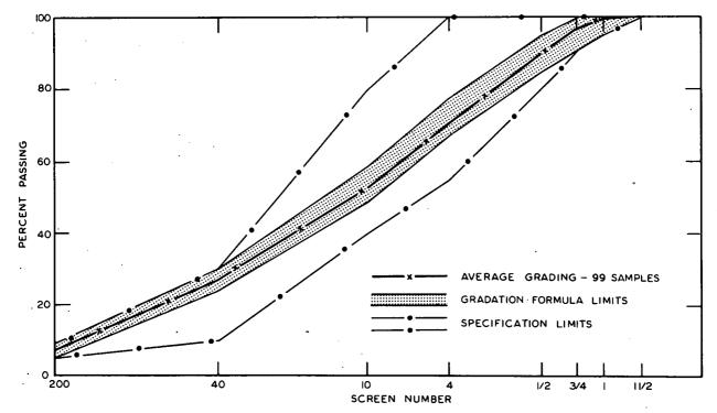
Figure 58. Gradation of subbase material in-place.
