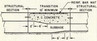
Figure 23. Details of transition pavement between structural sections.
