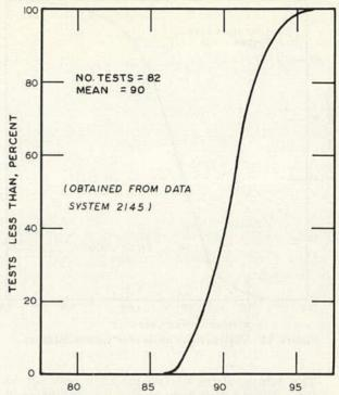
Figure 91. Penetration at 77 F of asphalt cement.
