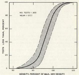
Figure 67. Subbase density after subgrading, rigid tangents.
