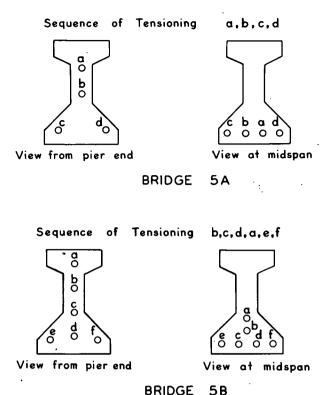
Figure 134. Tendon locations within post-tensioned beams.
