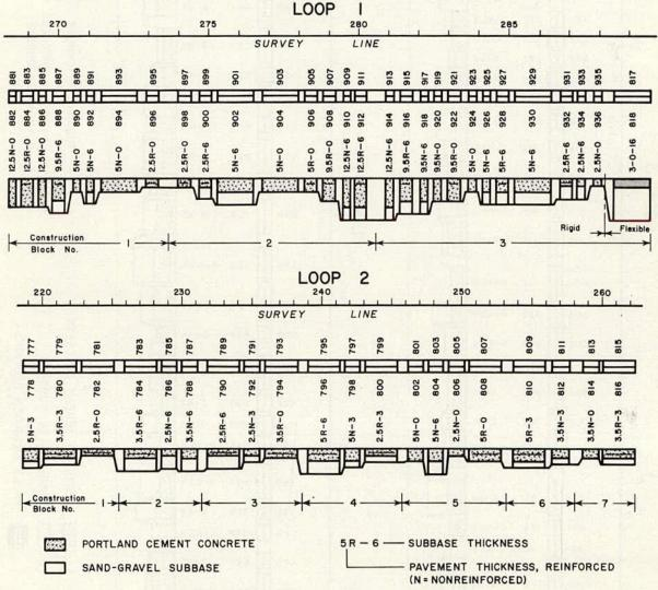
Figure 20. Layout of rigid tangent, Loops 1 and 2.
