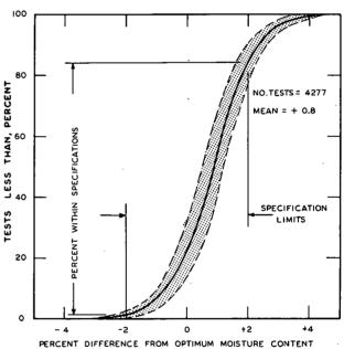
Figure 46. Constructed moisture content of embankment, rigid tangents.
