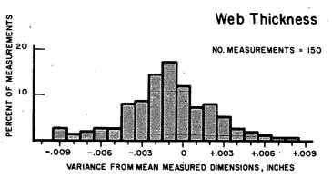
Figure 146. Measurements of WF steel I-beams.
