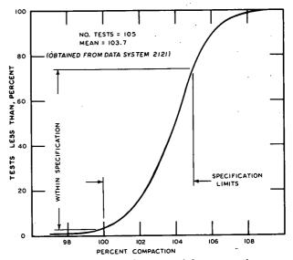
Figure 88. Gravel base, special—compaction.
