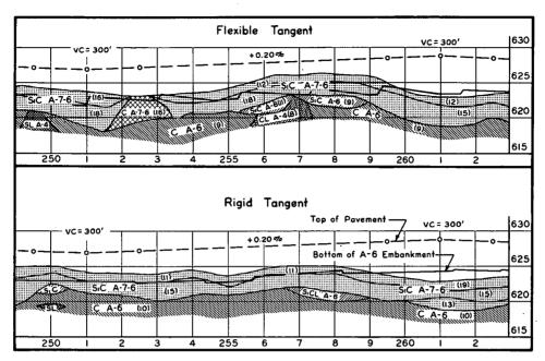
Figure 7. Existing soils profiles, Loop 5.
