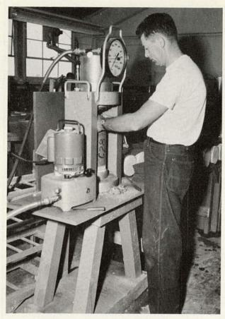
Figure 116. Testing concrete cylinders.
