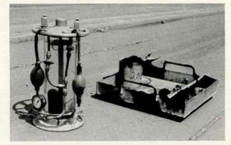
Figure 61. Volumeter used to measure volume of hole for field density test.
