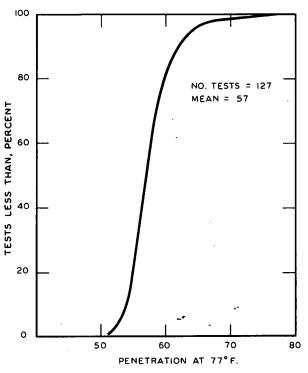
Figure 103. Penetration at 77 F on recovered asphalt cement.
