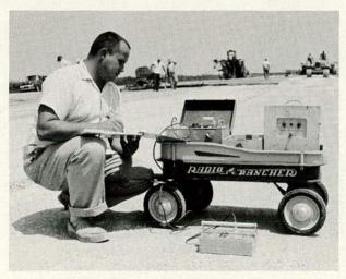
Figure 78. Determining field density of base with nuclear density equipment.
