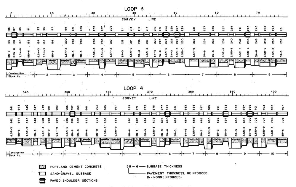
Figure 21. Layout of rigid tangent, Loops 3 and 4.
