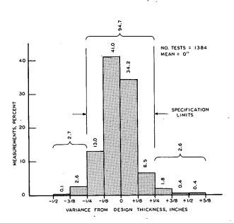
Figure 102. Asphaltic concrete surfacing thickness.
