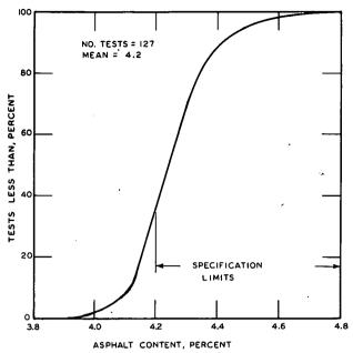
Figure 93. Extractions on binder course mixture.
