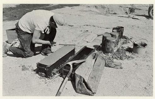
Figure 139. Preparing concrete test specimens.
