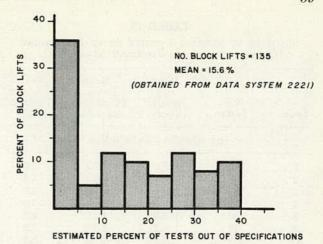
Figure 65. Subbase compaction, rigid tangent.
