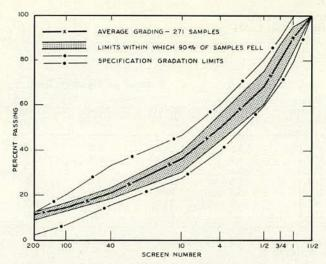
Figure 76. Gradation of crushed stone base, special—samples from road.
