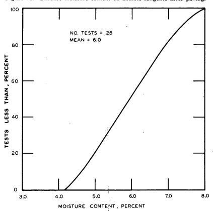
Figure 71. Subbase moisture content on rigid tangents after paving.
