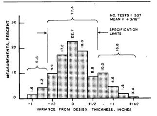
Figure 69. Subbase thickness, rigid tangents.
