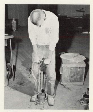
Figure 1-B. Obtaining Proctor needle reading on molded soil samples.
