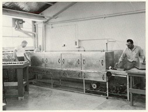
Figure 40. Continuous drying oven.
