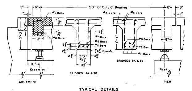
Figure 132. Details of reinforced concrete beam bridges.
