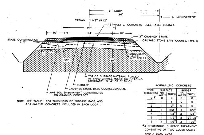
Figure 11. Cross-section details of flexible pavements on test tangents.
