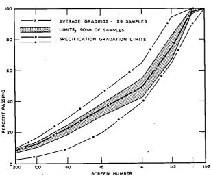
Figure 87. Gradation of in-place gravel base material.
