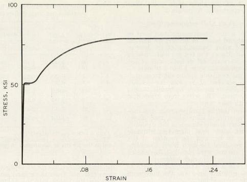
Figure 144. Typical stress-strain curve for reinforcing bars.
