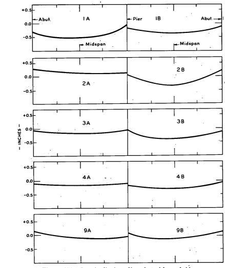
Figure 150. Longitudinal profiles of steel beam bridges.
