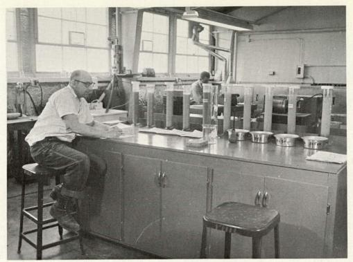
Figure 30. Testing embankment soil.
