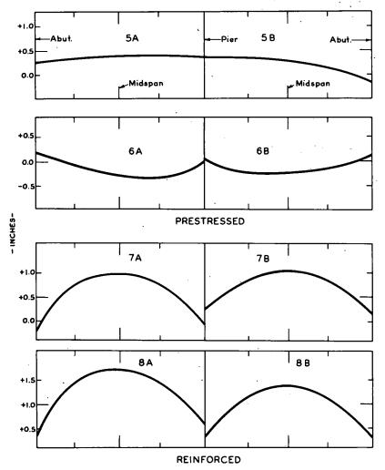
Figure 152. Longitudinal profiles of prestressed and reinforced concrete beam bridges.
