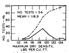
Figure 33. Tests on gray A-6 soil.
