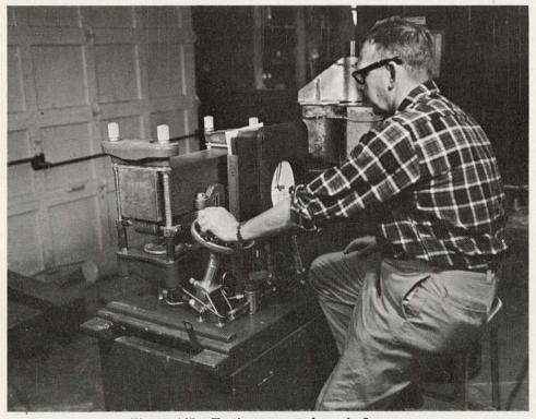
Figure 145. Testing concrete beam in flexure.
