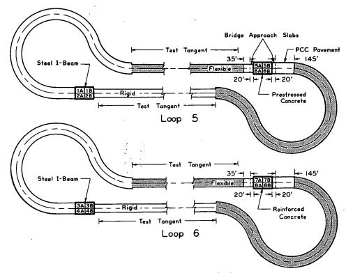
Figure 4. Locations of test bridges.
