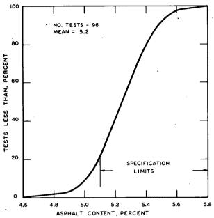
Figure 94. Extractions on surface course mixture.
