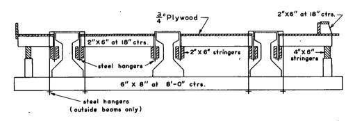
PRESTRESSED BEAM BRIDGES Figure 135. Forms for bridge decks.
