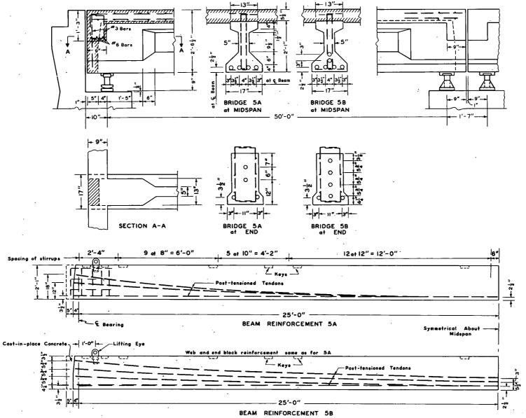
Figure 127. Post-tensioned beams.
