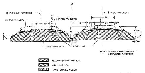
Figure 8. Typical cross-section of A-6 soil embankment with sand-gravel mulch cover.
