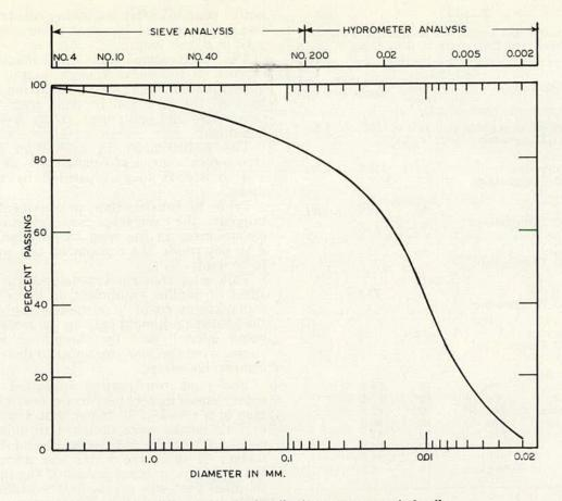
Figure 34. Grain size distribution curve, gray A-6 soil.
