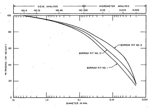
Figure 32. Grain size distribution curves, yellow-brown A-6 soil.
