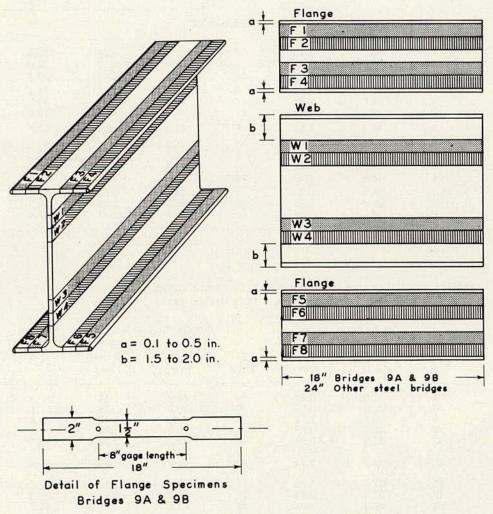
Figure 141. Tension coupons from WF beams.
