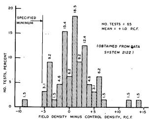
Figure 89. Field density, cement-treated base.
