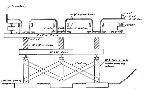
Figure 136. Forms and falsework for reinforced concrete beam bridges.
