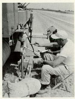
Figure 48. In-place CBR test on completed embankment.
