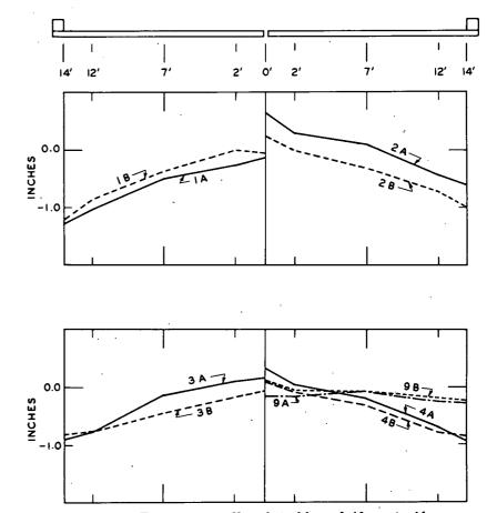
Figure 151. Transverse profiles of steel beam bridges at midspan.
