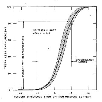
Figure 45. Constructed moisture content of embankment, flexible tangents.
