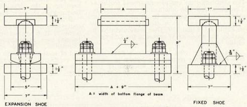
Figure 120. Details of bearing shoes.
