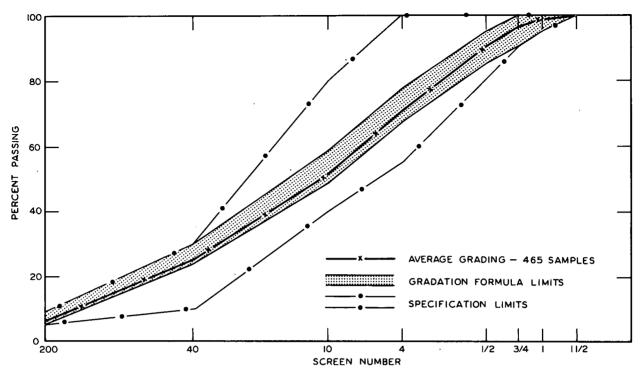
Figure 51. Gradation of subbase material.
