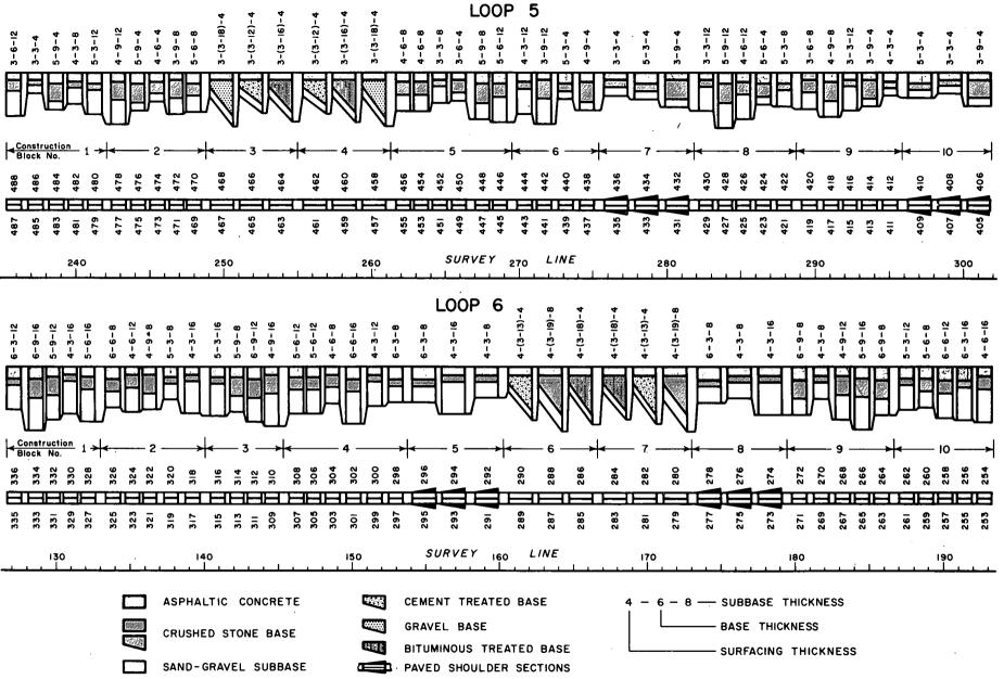
Figure 14. Layout of flexible tangent, Loops 5 and 6.
