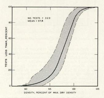
Figure 66. Subbase density after subgrading, flexible tangents.
