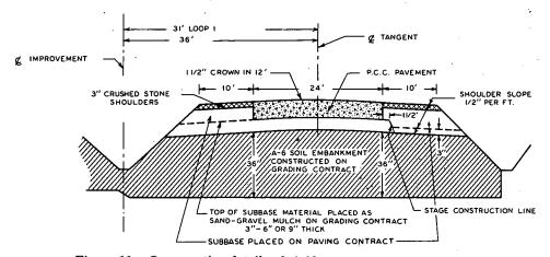
Figure 16. Cross-section details of rigid pavements on test tangents.
