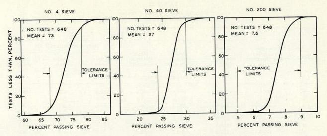
Figure 59. Gradation of subbase material in-place.
