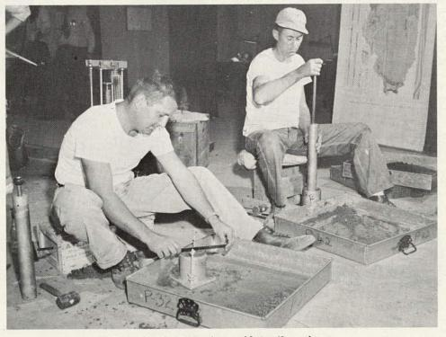
Figure 3-B. Preparing molded soil specimen.
