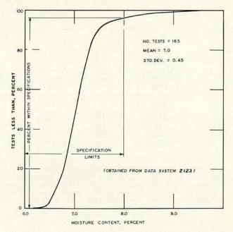
Figure 77. Moisture content of crushed stone base course, special.
