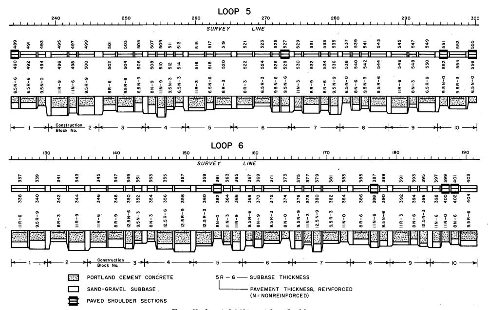
Figure 22. Layout of rigid tangent, Loops 5 and 6.
