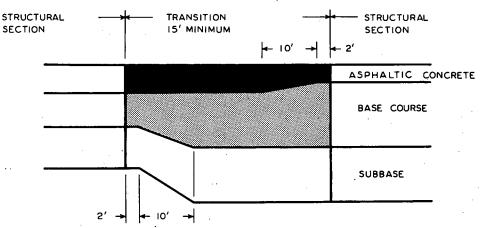
Figure 15. Details of transitions between structural sections.
