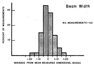
Figure 148. Measurements of reinforced concrete beams.
