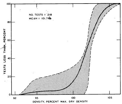
Figure 81. Crushed stone base density after subgrading.
