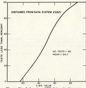
Figure 60. Laboratory CBR determinations on subbase material.
