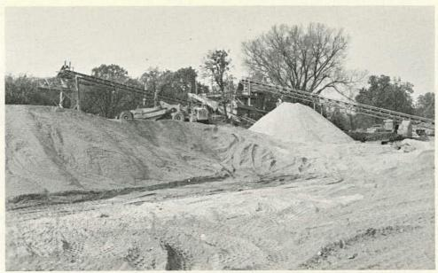
Figure 52. Washing and screening plant for subbase material.
