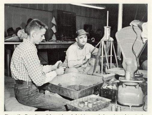
Figure 42. Extruding soil from tube and obtaining sample for moisture determination.
