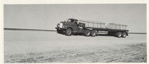
Figure 22. The loop turnarounds were superelevated at a rate of 0.2 ft per ft on the outer lane. All vehicles normally used this lane when traveling at 25 mph or faster.
