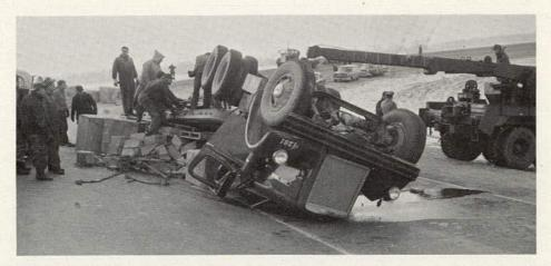
Figure 29. Several accidents such as this occurred on the loop turnarounds. The driver of this vehicle remained in the cab and was not injured despite the extensive damage to the vehicle.
