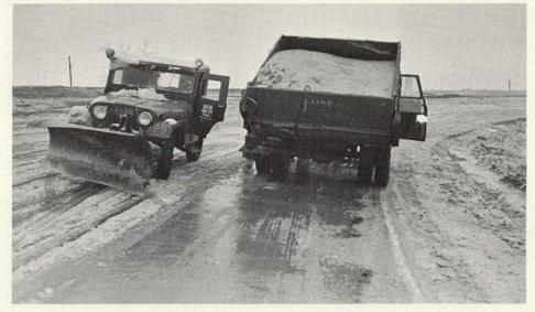
Figure 44. Salt and abrasives were used on the loop turnarounds to remove snow and ice and permit traffic operation.
