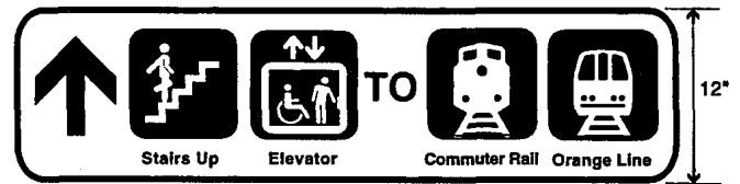
Figure 24. Straight ahead, up the stairs, or up the elevator to the commuter rail and Orange Line rapid rail platforms. Note: This sign is mounted on a wall at a height less than 80 in. (2,032 mm), thus the arrow points "up" and means straight ahead.
