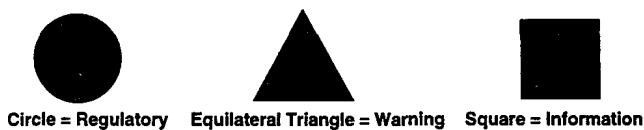
Figure 3. Geometric shapes used by designers to represent the regulatory, warning, and information categories of signs.
