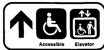
Figure 25. Straight ahead via an accessible route to the elevator. Note: This sign is also mounted on a wall at a height below 80 in. (2,032 mm), thus the straight ahead arrow is pointing "up."
