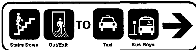
Figure 29. Down the stairs, out of the station to taxi stands and bus bays to the right. Note: The arrow on the right points to the right and pulls the symbols.
