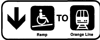
Figure 27. Straight ahead via an accessible ramp to the Orange Line rapid rail platforms. (Note: This sign is mounted overhead higher than 80 in. (2,032 mm) so the straight ahead arrow is pointing "down.")
