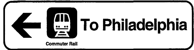
Figure 31. Left to commuter rail platform to catch the commuter train to Philadelphia. Note: The arrow and the text "To Philadelphia" are centered on the horizontal centerline of the sign board.
