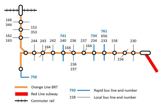
Rail services typically rely on feeder bus service to some degree—less so for urban subway and AGT systems supplemented by surface bus routes and more so for light rail and commuter rail lines, particular in suburban areas. Many South American BRT systems use a feeder service pattern (*36*).
