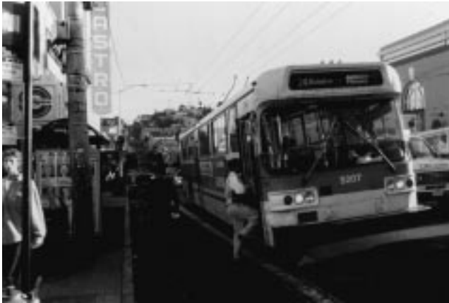
Figure 2-5. Before MUNI added bus bulbs or nubs along 17th Street, buses often stopped in the street to pick up passengers.
