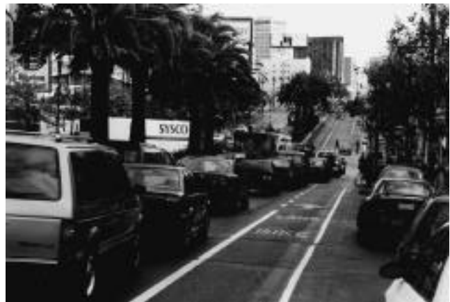
Figure 3-10. The transit signal priority system on Upper Market Street allows for passenger boarding during the red cycle of the traffic light (above), while causing little delay to cars traveling in the shared transit lane (below).
