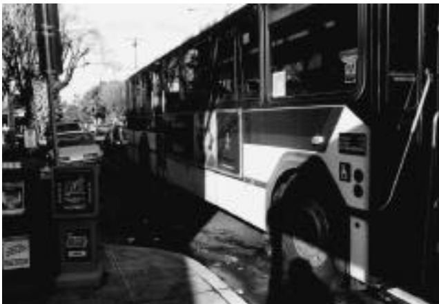
Figure 3-3. Curb extensions were added to NW 23rd Avenue to reduce illegal passing of loading buses by cars (above). Although the extensions are the length of a full-sized bus, when transit amenities block the sidewalk many drivers do not pull up all the way, which forces alighting passengers to disembark into the street (below).
