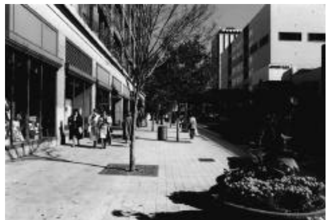
Figure 3-5. In the late 1980s, Rochester's Main Street was narrowed to four lanes, which provided room for widened sidewalks and extensive streetscape enhancements.
