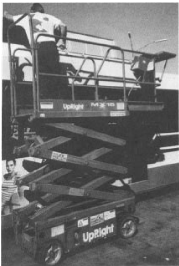
Figure 2.7 A Powered Work Platform for Maintenance of Components Located in the Roof Area
