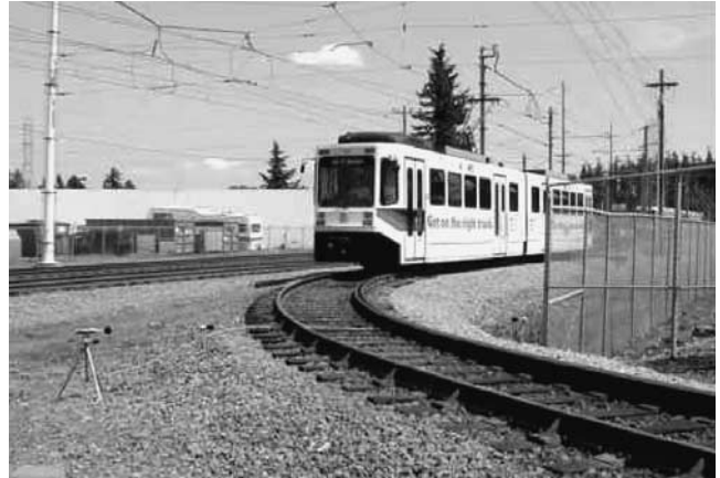
Figure 4. Noise data microphones located on test curve.
