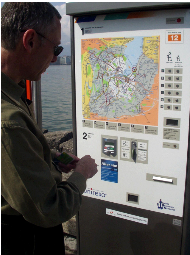
Figure 11. The Unireso ticket vending machine: the card is inserted, a fare is selected, the card is pulled out, and a paper ticket showing the valid zone and fare period is dispensed.
