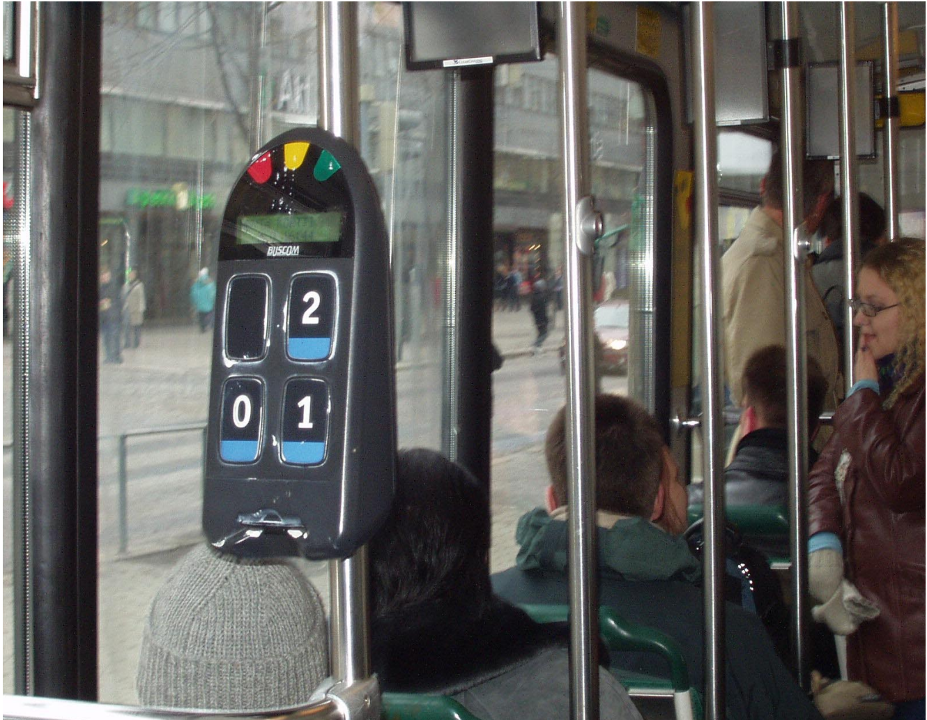
Figure 13. A customer smartcard fare reader on a trolley in Helsinki. The card reader portion is located in the center of the unit, between the 0 and the 2. The numbers are pressed to validate various types of service. A customer readout screen is directly above the numbers. On top are three different lights that flash a specific color depending on whether a card has worked successfully or has sufficient value.
