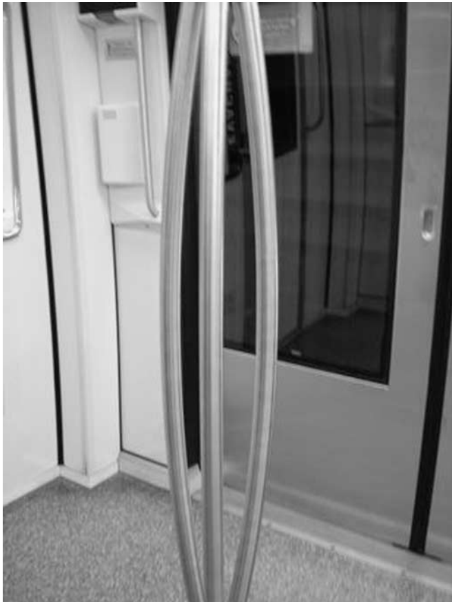
Figure 11 The three-pole stanchion provides more space for standees to hold.
