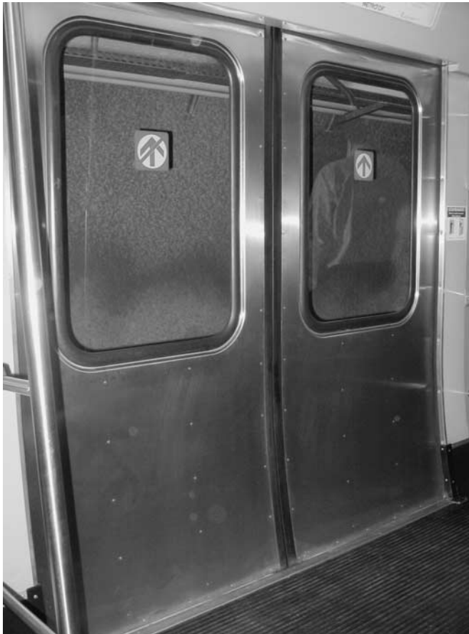
Figure 3 and 3a Signage to reduce the conflict between boarding and alighting passengers in Brasília.
