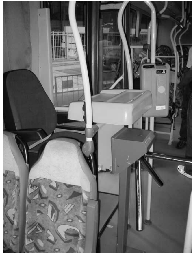
Figure 15 A conductor position and turnstiles on board an articulated bus.
