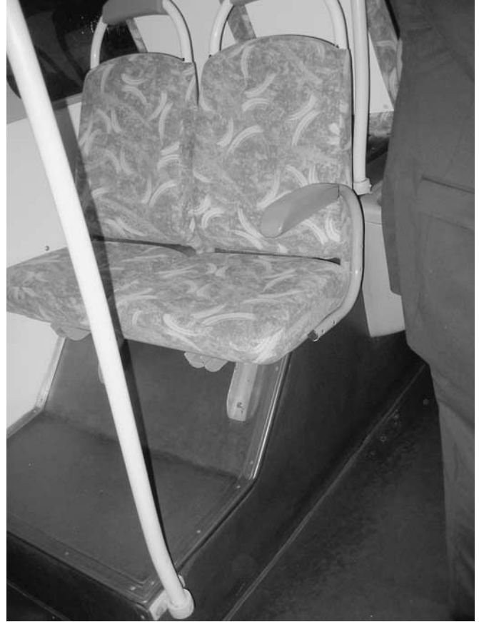
Figure 12 Seats mounted on the large wheel wells in low-floor buses.
