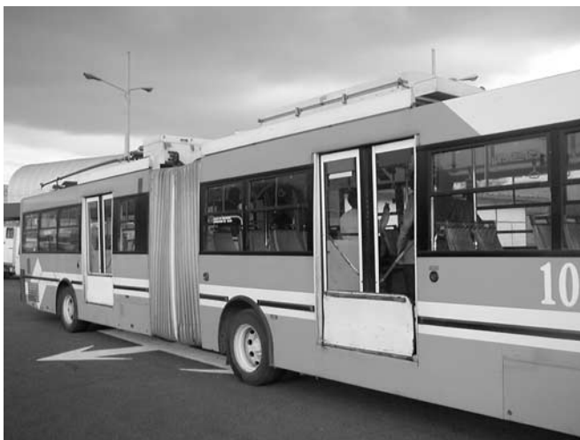
Figure 5 Raised boarding platforms in front of the exit doors of the articulated Trolebús.
