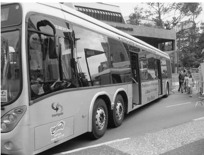
Figure 14 and 14a A bus built with two doors on each side and three axles.
