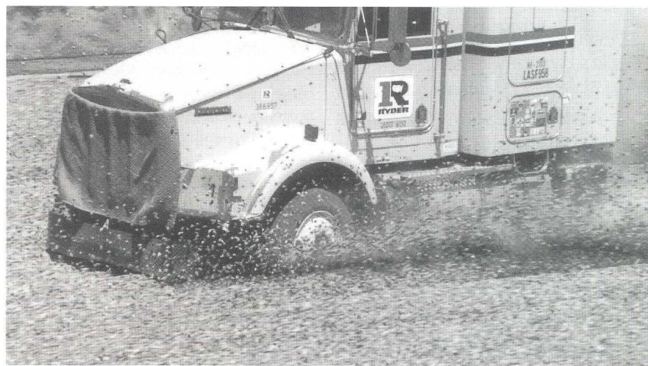
Aggregate sprays as arrester bed slows truck.
