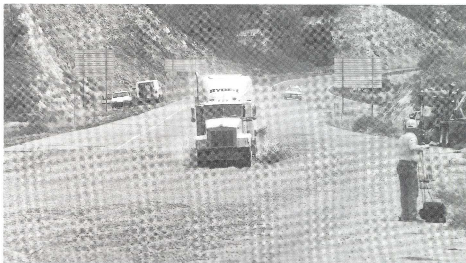
Arrester bed entry shows truck, pilot vehicle behind, and extraction vehicle to right.
