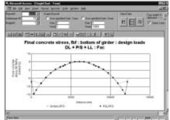
FIGURE 1 Computer program compares final concrete stresses from Pennsylvania DOT Prestressed LRFD and Wyoming BRASS Girder LRFD.
