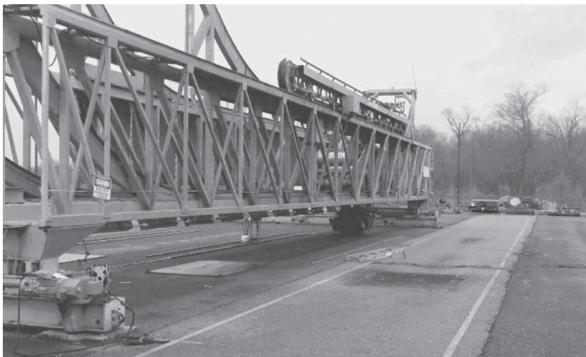
Accelerated loading facility device at Louisiana Transportation Research Center's Pavement Research Facility, Port Allen.
