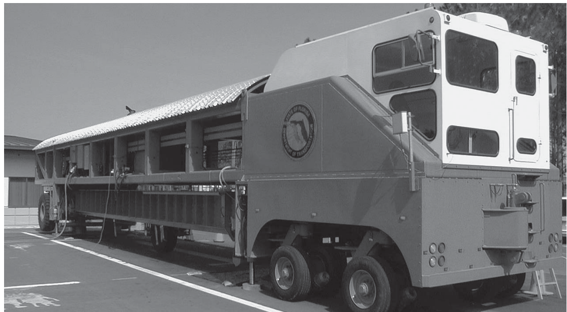
Heavy vehicle simulator at new State Materials Research Park in Gainesville, Florida, applies equivalent of 20 years of vehicle loads in only 3 months.
