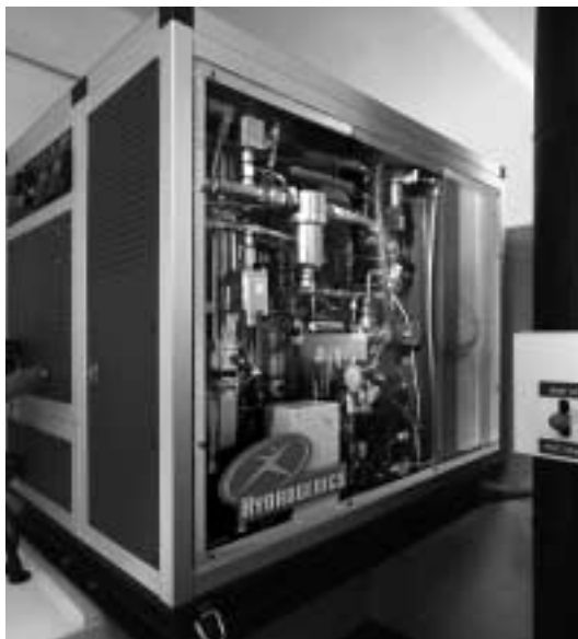
GM diesel hybrid can switch to auxiliary power from hydrogen fuel cell.
