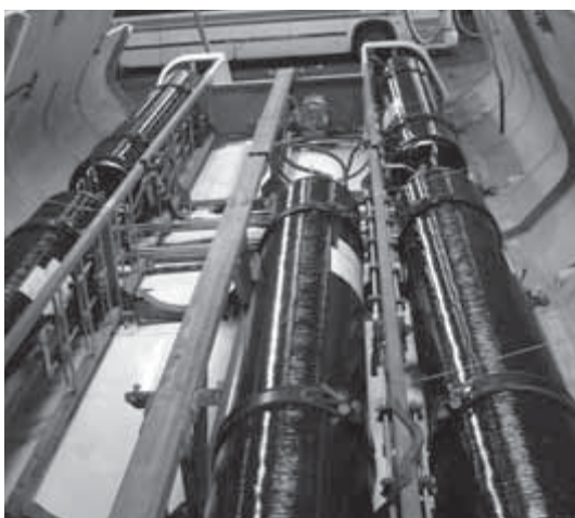
CNG fuel cylinders, fuel lines, and safety devices under bus roof.
