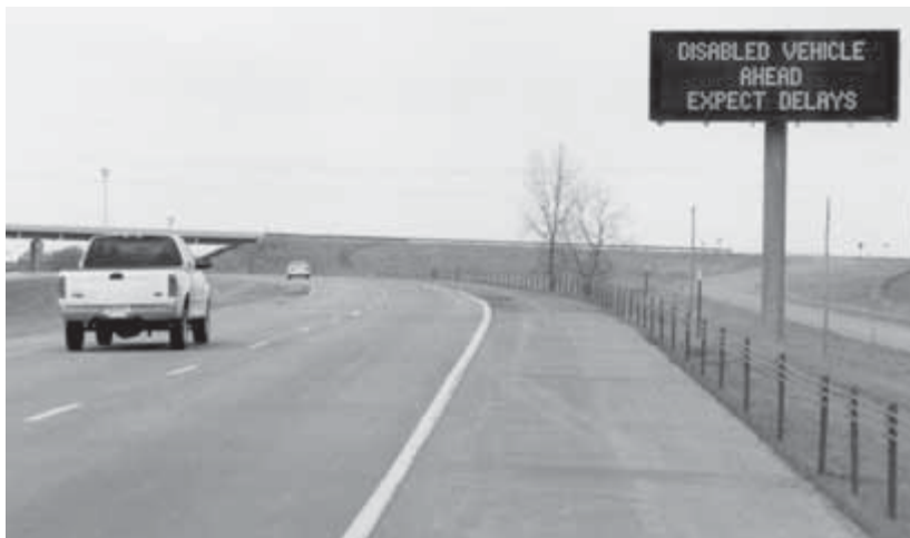
The National Transportation Communications for ITS Protocol (NCTIP) for Dynamic Message Signs was among the applications areas discussed by the study committee. Above, an NCTIP-compliant variable message sign near Sioux Falls, South Dakota.
