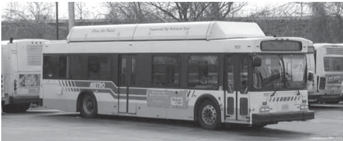
CNG-powered bus in Akron (Ohio) Metro system; the CNG fuel cylinders are mounted on the bus roof, beneath the housing.
