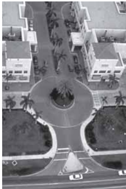
PHOTO: DAN BURDEN, WALKABLE COMMUNITIES, INC. Roundabout and vegetation median calm traffic in Boca Raton, Florida.
