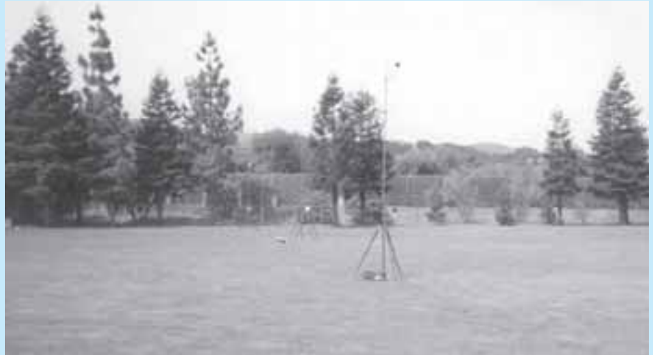
Microphones and sensors measuring traffic noise.
