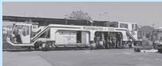
BART railgrinder used to reduce noise levels.
