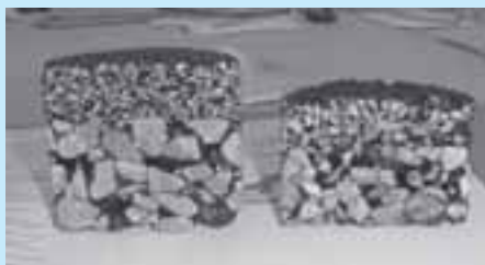
Core samples of double- and single-layer porous asphalt from Denmark.
