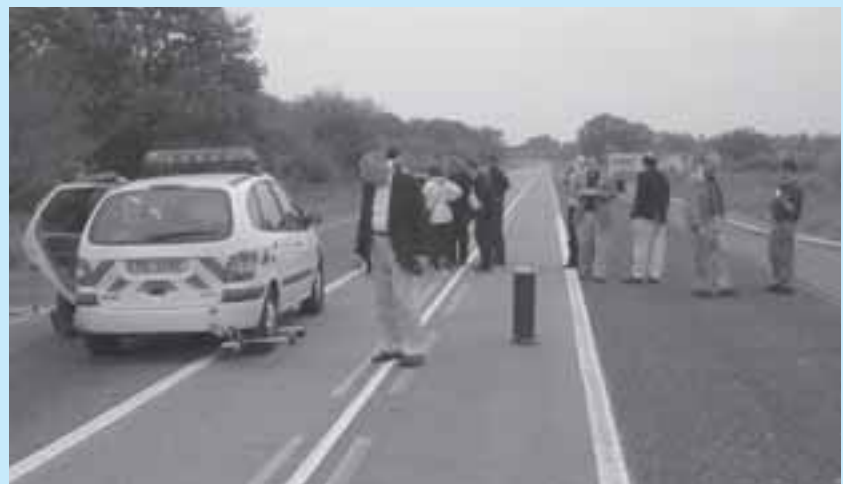
Scan group inspects the sound intensity setup on light vehicle at French test track.
