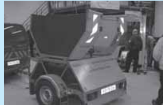
Trailer used in the Netherlands for sound measurement by the close-proximity method.
