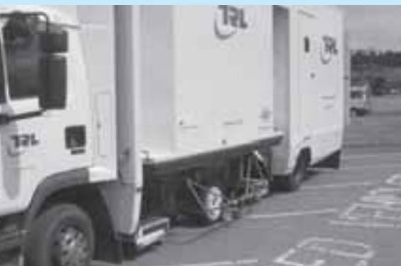
In the United Kingdom, TRITON uses a sound intensity setup on a heavy vehicle that can vary loading to the wheel, in line with tire tracks.
