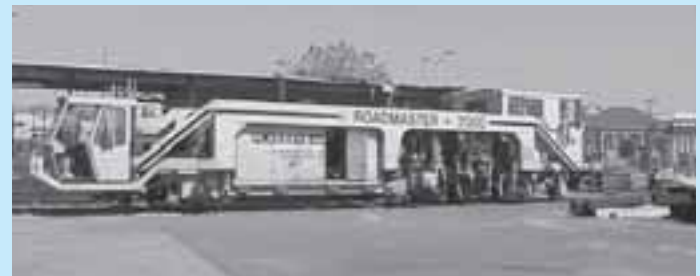
BART railgrinder used to reduce noise levels.
