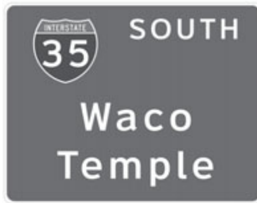
FIGURE 2 Clearview version of guide sign increases legibility at greater distances without increasing letter or sign sizes.
