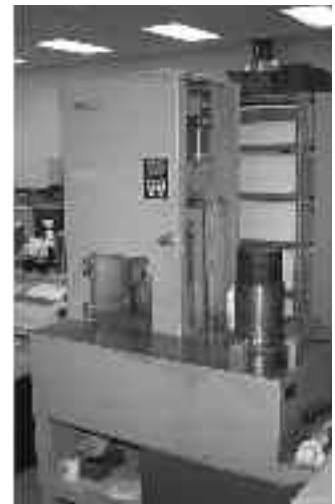
Superpave gyratory compactor, which prepares loose HMA mixtures for a variety of laboratory tests.
