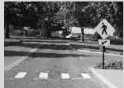
A road safety audit identified a crosswalk (left) not visible to approaching motorists. A sign was installed to indicate the location of the crosswalk clearly (right) and to enhance pedestrian safety.
