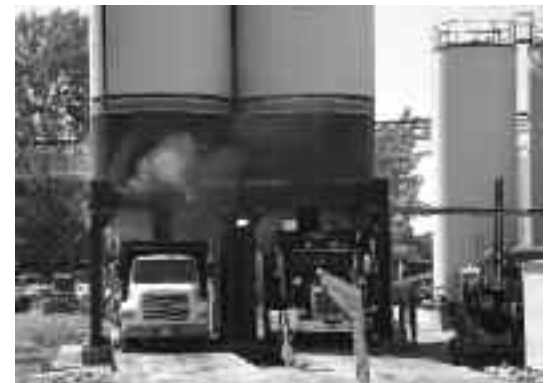
Demonstration of warm-mix asphalt paving ( left ). Warm-mix asphalt mixtures can be manufactured at production facilities with reduced emissions and decreased energy use.
