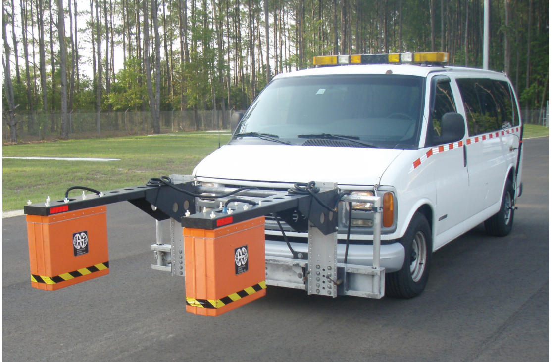
Survey vehicle equipped with ground-penetrating radar.
