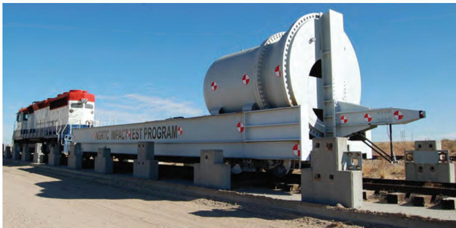
Full-scale tank car impact test setup for evaluating safety improvements under the Next-Generation Railroad Tank Car project at the Transportation Technology Center near Pueblo, Colorado.
