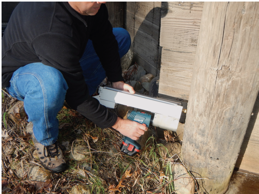
A resistance microdrill is the preferred drilling inspection technique for timber bridge elements.
