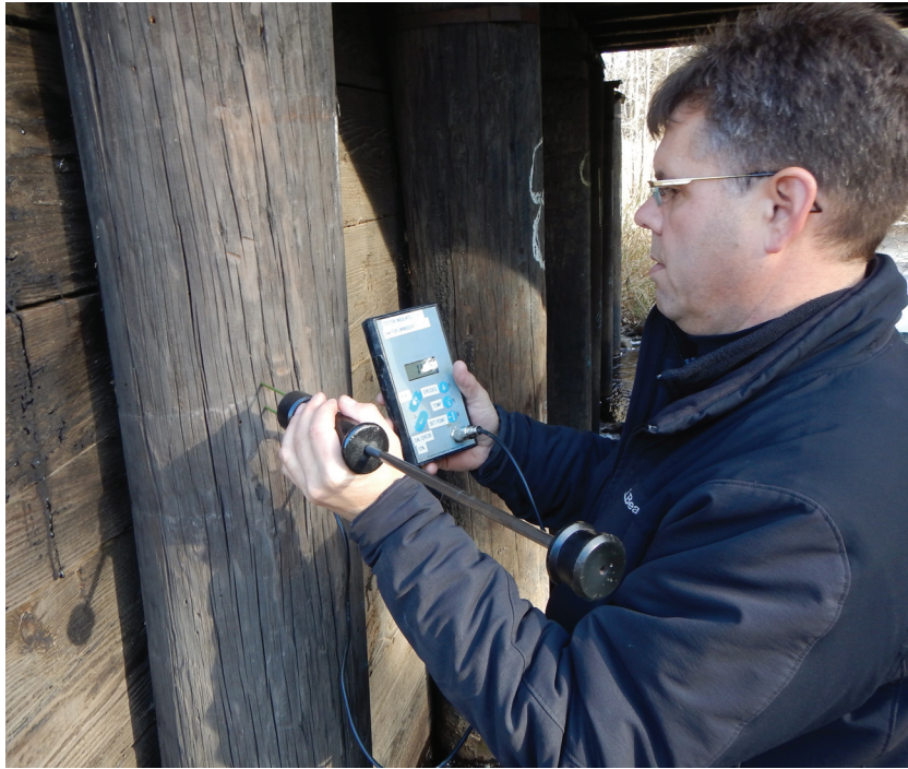
A pin-style moisture meter is used to determine the moisture content of timber elements.
