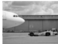
Towbarless tractor after disengaging from an aircraft nosewheel.
