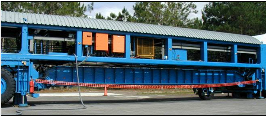
Accelerated Pavement Testing
