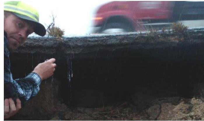
Figure 4.3-5 - Bridging in Flexible Pavements
