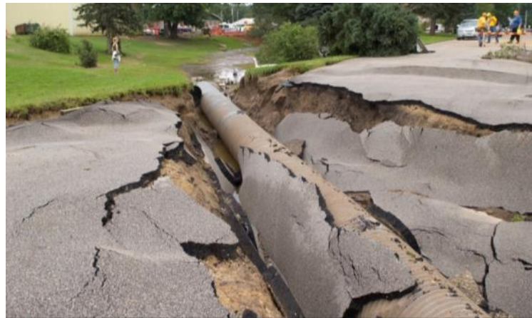
Figure 4.3-6 – Failure Due to Piping (Water flowing along outside of pipe and washing away backfill)
