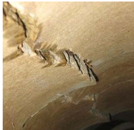
Figure 4.10-3 – Cracks with Radial Offset
