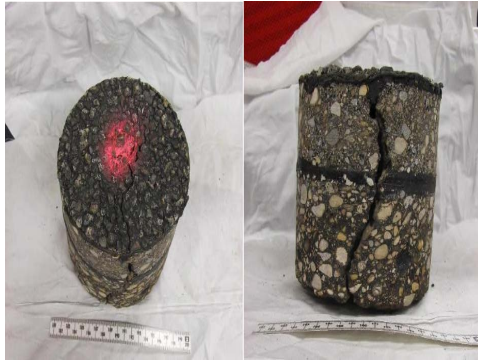
Chip seal with crack filling
