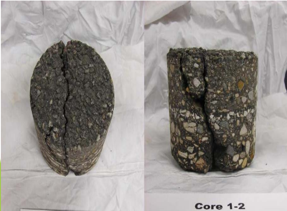
Chip Seal without crack filling
