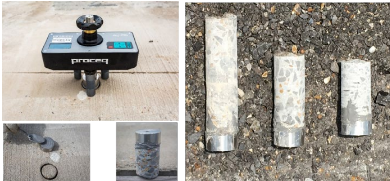
Figure: Pull-off Test of COA Sections
