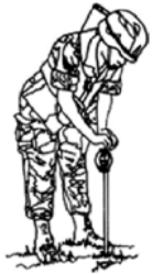
Using the cone penetrometer in the upright position.
