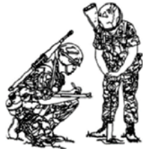
Measuring cone index in the remolding cylinder before and after hammer blows.
