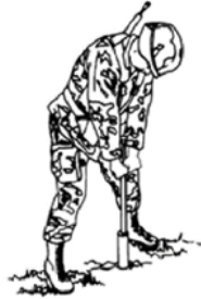
Using the sampler to obtain a soil sample for a remolding test.
