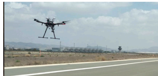
UAS used to inspect grounded aircraft after adverse weather events
