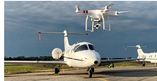
UAS used to inspect grounded aircraft after adverse weather events
