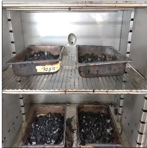
Laboratory mixture aging at 85°C and 135°C
