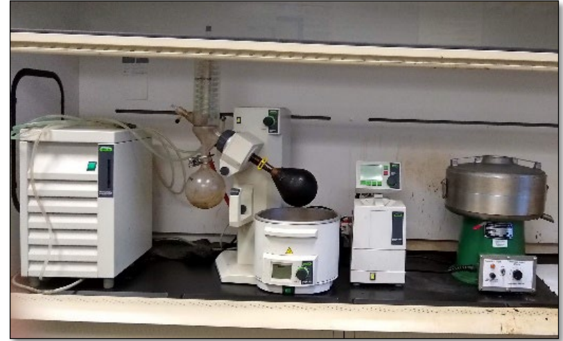
Asphalt binder extraction from loose mixture
