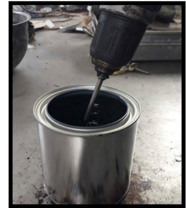
Mixing of SBS with asphalt binder by a hand drill
