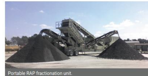
Portable RAP fractionation unit.
