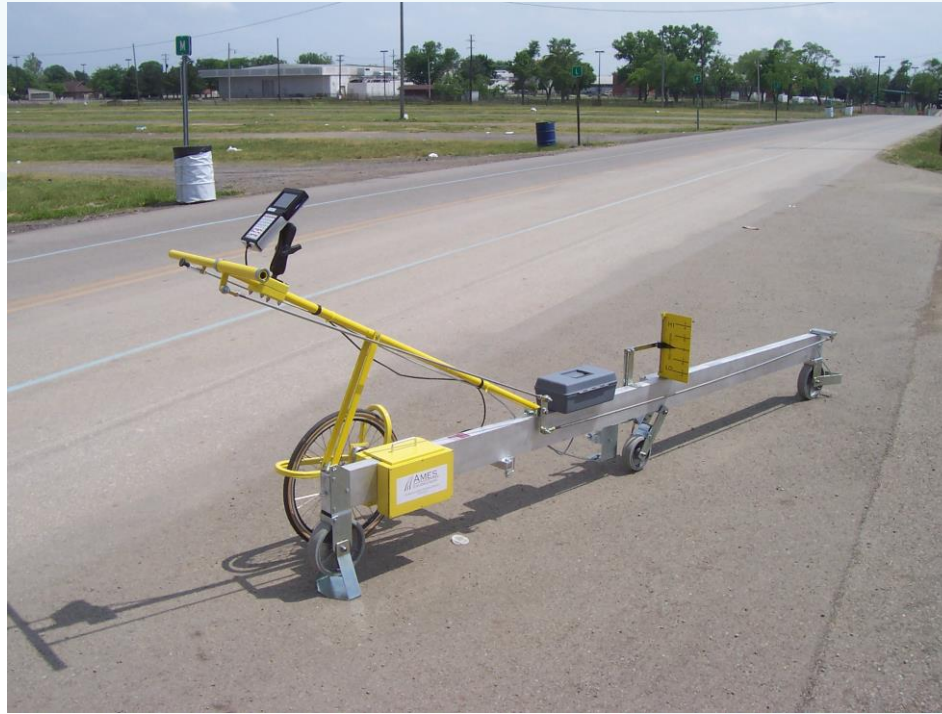
10-foot Rolling Straightedge, 1/8" Deviation
