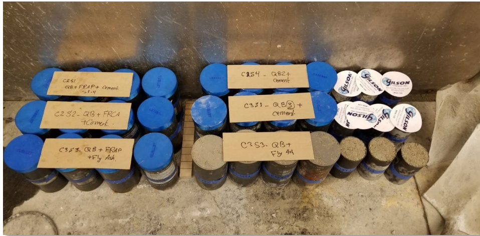
Molding of Samples (4" x 8" cylinders)
