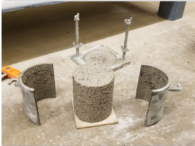
Sample Preparation Using a Split Mold
