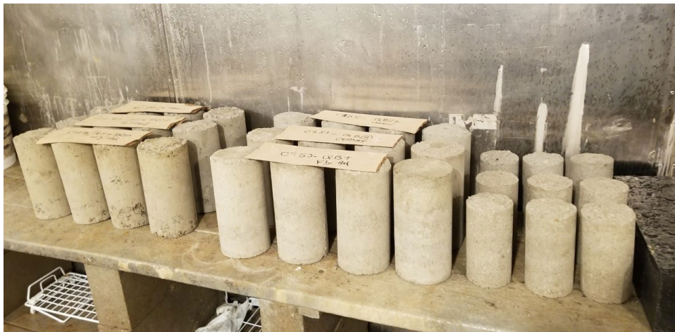
Moist Room Curing (7 days)
