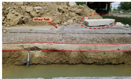
C3S2W – QB2 + Cement Subbase + CA06_R
