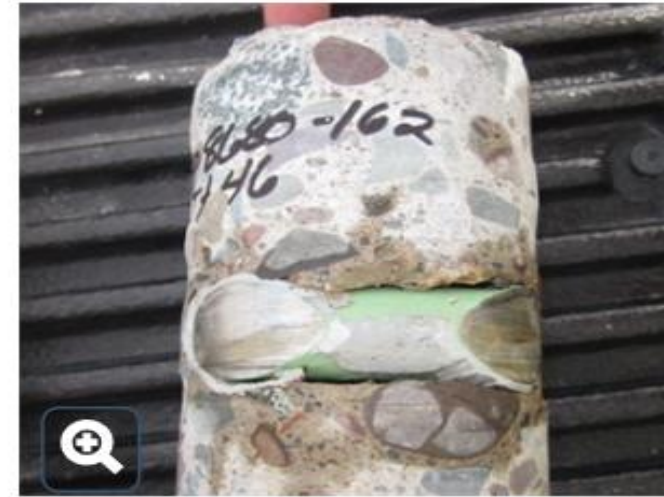
Unacceptable Epoxy Adhesive Coverage
