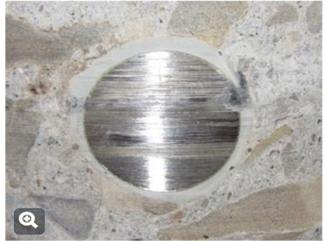
Acceptable – Epoxy Adhesive
