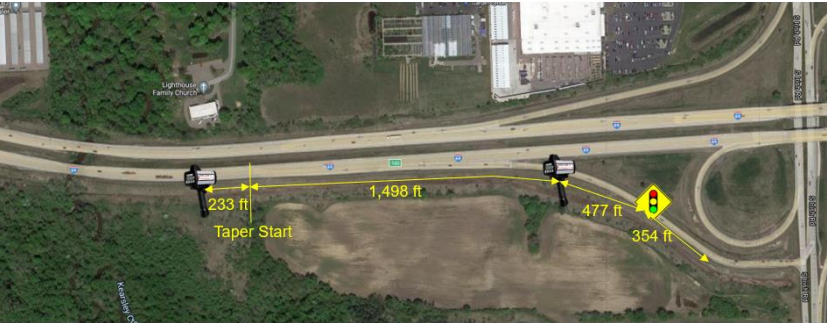
Diamond, parallel exit ramp
