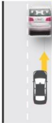
Stationary balloon car: Stationary dummy vehicle -tests run at 12 and 25 mph
