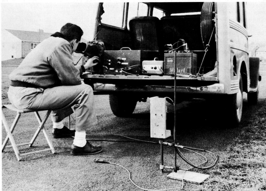
Figure 2. Measuring pulse velocity with portable field unit.
