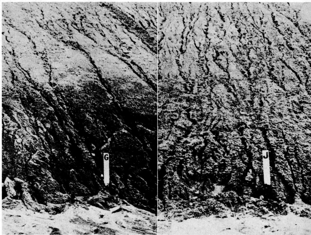
Figure 7. A CRD-189 surface-treated slope (at left) and a control slope (at right) illustrate effects of frost action on erosion.
