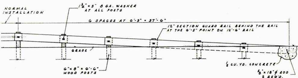
Figure 18. Guardrail sloped end treatment.
