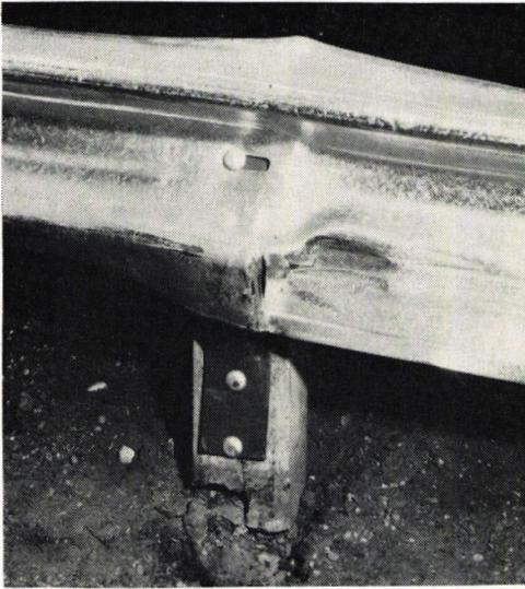
Figure 11. Flattened and torn guardrail ribbon.
