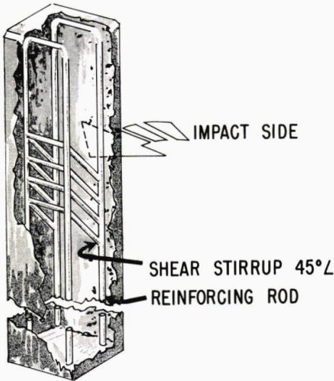
Figure 4. Construction of 6-by 8-in. concrete post.
