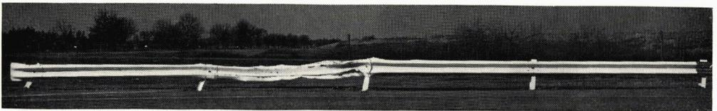
Figure 21. Post movement after impact on short section of guardrail.
