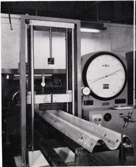
Figure 9. Beam test of guardrail ribbon.
