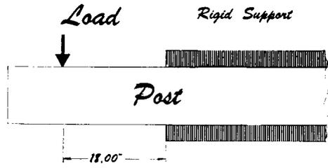
Figure 2. Post breaking fixture.
