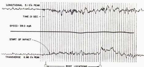
Figure 15. Oscillograph of guardrail impact.
