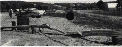
Figure 22. Result of impact on sign protection guardrail.
