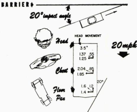
Figure 23. Peak accelerations during impact.
